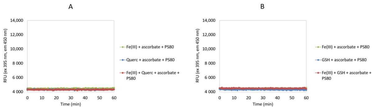
**Figure S5.** Time courses of the production of  $\cdot\text{OH}$  (RFU, relative fluorescence units) during autooxidation of Fe(III) complexes measured according to the fluorescence intensities of 7-hydroxycoumarin-3-carboxylic acid after incubations of CCA with ascorbate and PS80  $\pm$  Fe(III), and  $\pm$ quercetin (Querc) **(A)** and  $\pm$  glutathione (GSH) **(B)** (see also Figure 2 for EDTA/DTPA).
