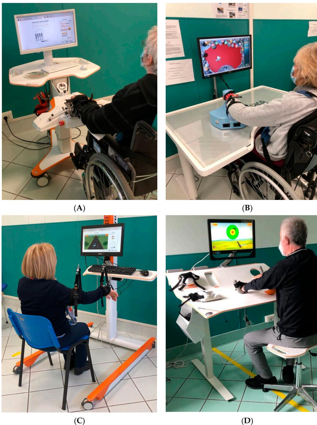
**Figure 1.** Robotic and sensor-based devices used to treat the upper limb: (A) Amadeo (Tyromotion); (B) Motore (Humanware); (C) Diego (Tyromotion); and (D) Pablo (Tyromotion).
