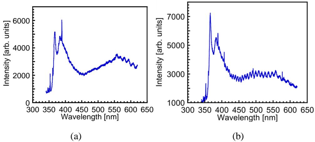
**Figure S2.** PL spectrum for InGaN/GaN heterostructures grown on HEMT templates at the temperature of (a) 760 °C and (b) 780 °C.
