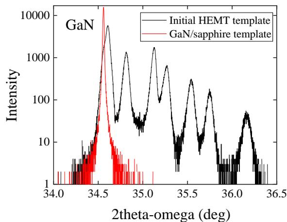
**Figure S1.** XRD 2theta-omega scan of the (002)-plane for the initial high electron mobility transistor (HEMT) template and GaN/sapphire template.
