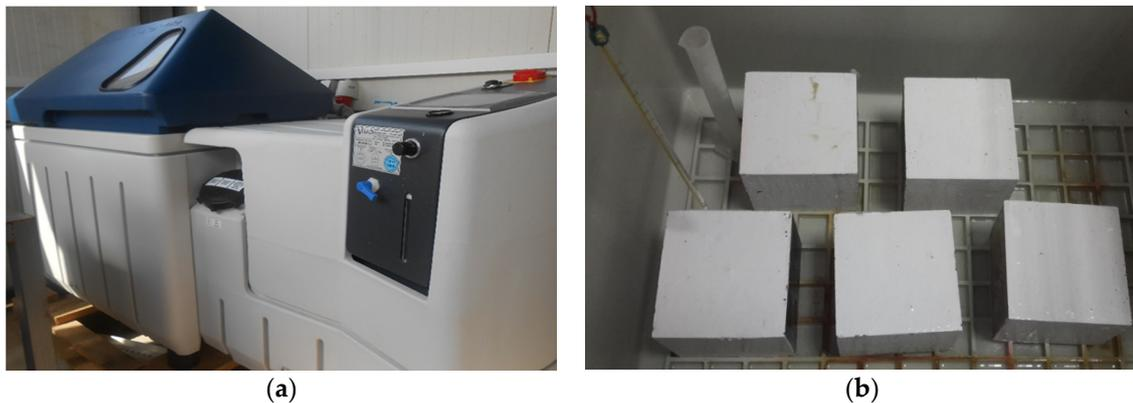
**Figure 2.** (a) Salt spray chamber and (b) sealed specimens inside the chamber.
