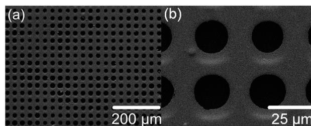
**Figure 4.** SEM images of a Kapton filter after heating at 350 °C for 10 min. The magnifications are (a) 200 $\times$  and (b) 1500 $\times$ .
