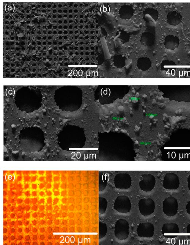
**Figure 2.** SEM images of a Kapton filter operated for 7 days. Micro dust is captured at the surface and around the pores. The magnifications are (a) 200 $\times$ , (b) 900 $\times$ , (c) 1500 $\times$ , and (d) 2900 $\times$ . Representative dimensions of the PM are shown in (d). (e) Optical microscope and (f) SEM images of a Kapton filter washed with tap water after filtration.
