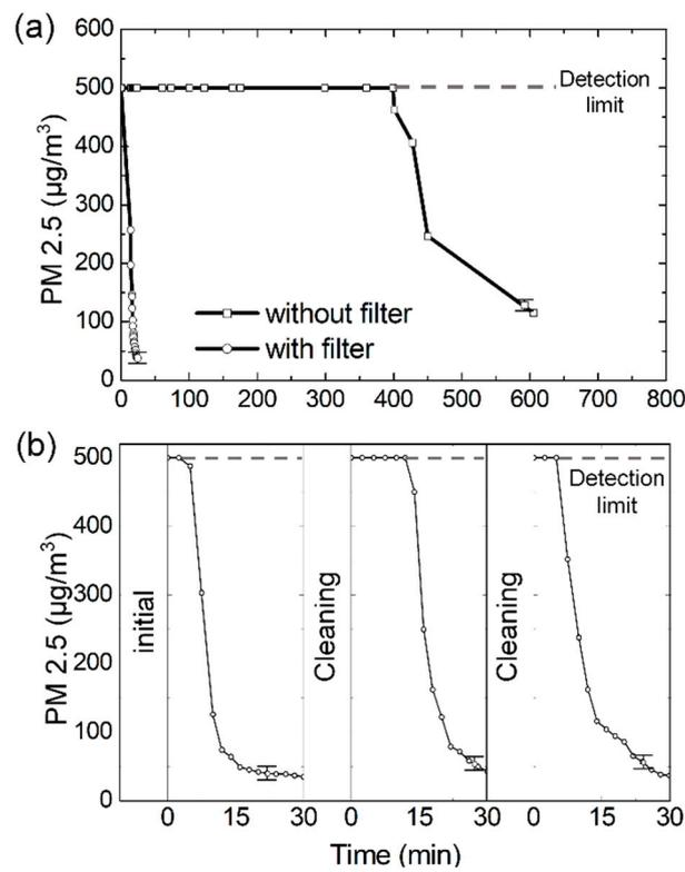
**Figure 3.** (a) Evolution of PM<sub>2.5</sub> density as a function of time with and without the Kapton air filter. The detection limit was 500  $\mu\text{g}/\text{m}^3$ . (b) The reliability and durability of the Kapton air filter after repeated washing.
