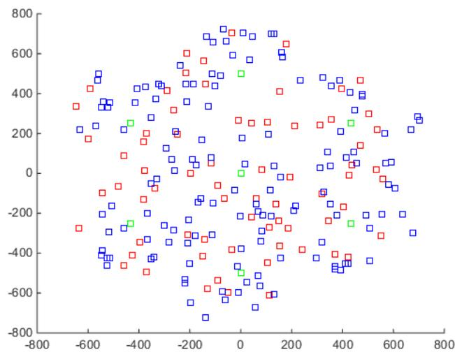
Figure 5. Hierarchical heterogeneous network model (7 macro cells, 70 micro cells, 140 users).
