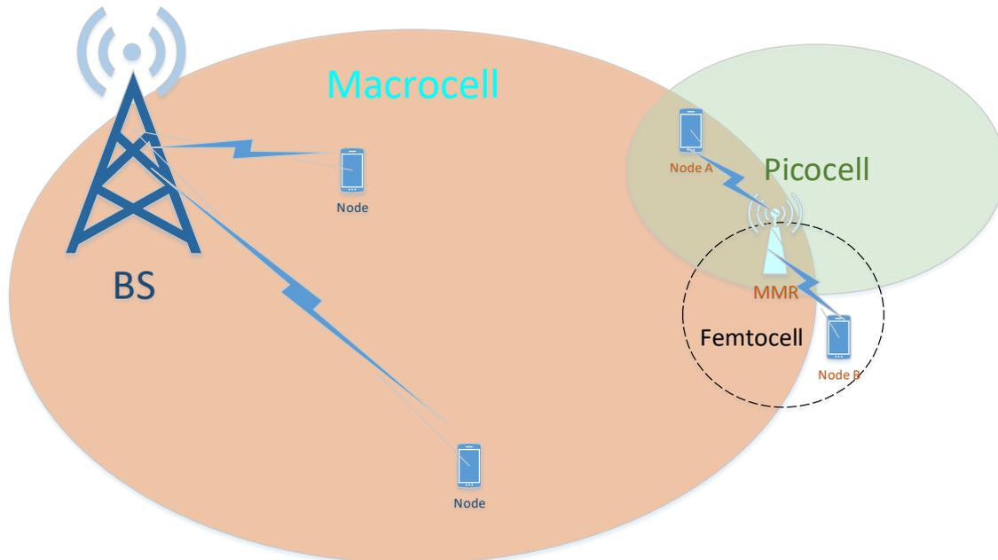
**Figure 1.** Multi-mode relay (MMR) running in the modes of picocell BS and femtocell BS.
