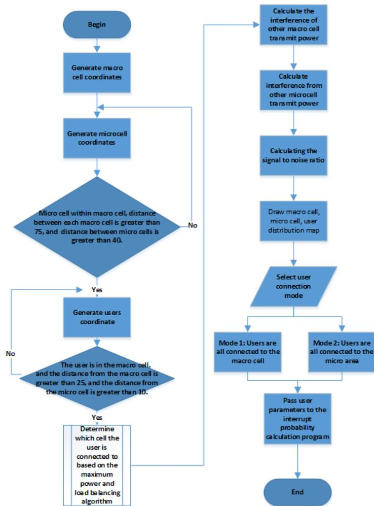
Figure 4. System simulation diagram.
