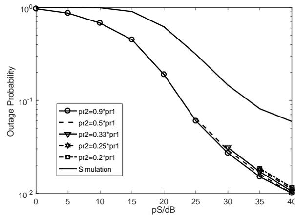
**Figure 7.** Outage probability of HHWN with MMR as different relay power  $p_{r2}$  equals 9/10,1/2,1/3,1/4,1/5 times  $p_{r1}$ .
