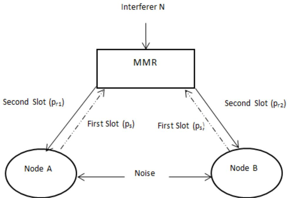
Figure 3. System model of multi-mode relay  $p_{r1} \neq p_{r2}$ .
