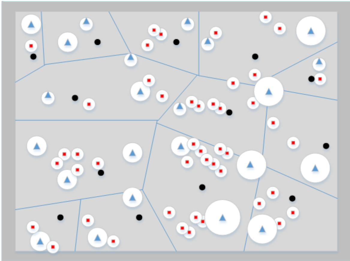
Figure 2. 3-tier HHWN max SINR downlink coverage regions with macrocells, picocells, and femtocells.
