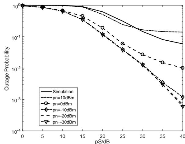
**Figure 9.** Outage probability of HHWN with MMR as different noise power  $p_n = \sigma_E^2 = 10 \text{ dBm}, 0 \text{ dBm}, -10 \text{ dBm}, -20 \text{ dBm}, -30 \text{ dBm}$ .
