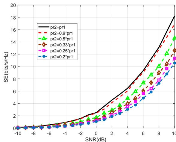
**Figure 8.** Spectral efficiency of HHWN with MMR as different relay power  $p_{r2}$  equals 9/10,1/2,1/3,1/4,1/5 times  $p_{r1}$ .
