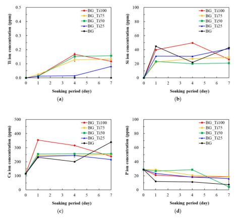
**Figure 4.** The ions released into SBF after the immersion of bioceramics composed of silica and titanium oxide with various concentrations of titanium oxide for 7 days, measured using ICP-MS. (**a**) Ti ion concentrations; (**b**) Si ion concentrations; (**c**) Ca ion concentrations; and (**d**) P ion concentrations.
