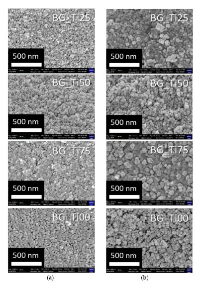
**Figure 1.** The microstructures of bioceramics composed of silica and titanium oxide with various concentrations of titanium oxide soaking in simulated body fluid (SBF) for (**a**) 0 days and (**b**) 7 days.
