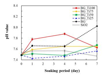
**Figure 3.** The pH value of SBF after the immersion of bioceramics composed of silica and titanium oxide with various concentrations of titanium oxide for 7 days.
