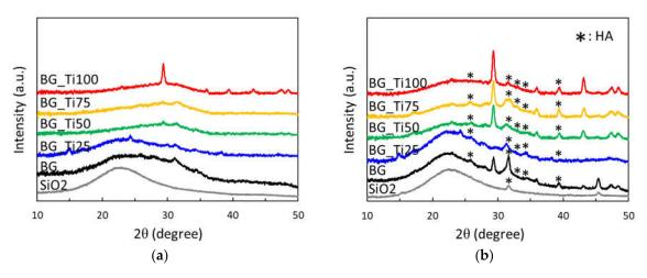
**Figure 2.** Phase identification by XRD of bioceramics composed of silica and titanium oxide with various concentrations of titanium oxide soaking in SBF for (**a**) 0 days and (**b**) 7 days.
