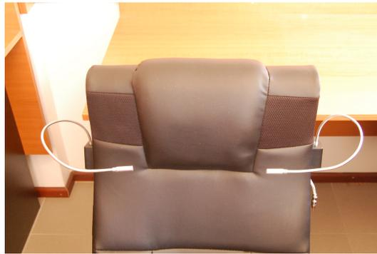
**Figure 13.** Photo of the headrest with the error microphones.
