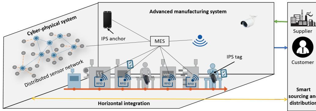
**Figure 3.** Intelligent Space (iSpace)-based integrated sensor signals can be used to monitor the work of the operators, extract their tacit knowledge, synchronize activities and provide contextualized information.
