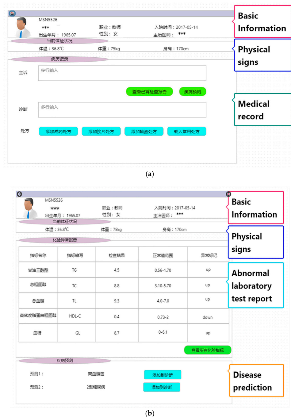
Figure 7. Two screenshots of the developed system using COCOA-RE approach: (a) the main work interface for clinicians; (b) the interface for viewing the laboratory test report.
