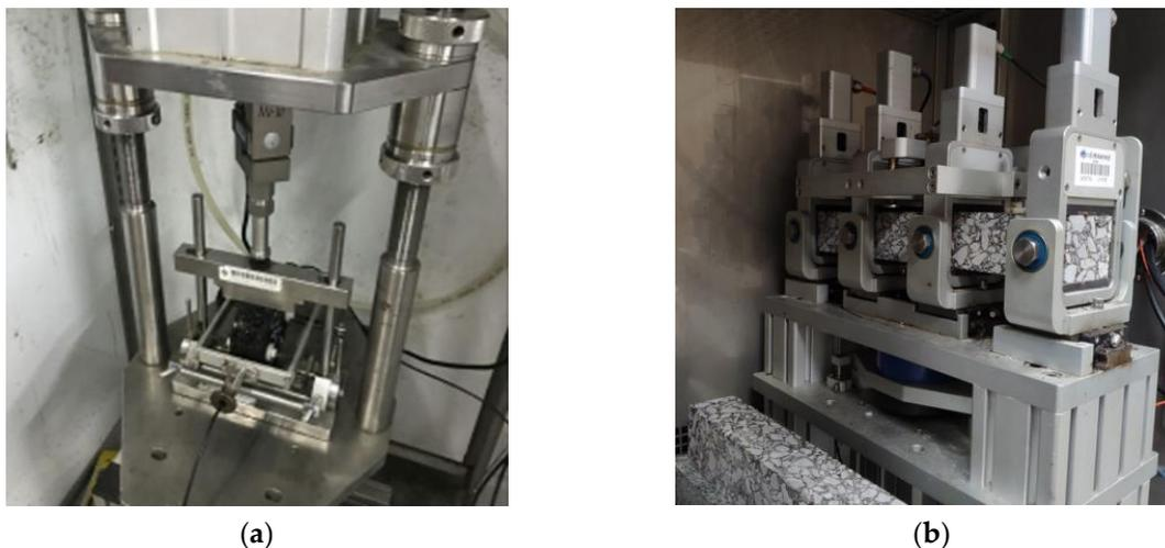
**Figure 2.** Fatigue characterizing tests: (a) indirect tensile fatigue test (ITFT) test for mixtures; (b) 4PB test for mixtures.
