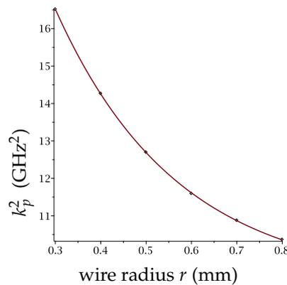
**Figure 6.** To design the required radius modulation, we need to know the variation of the effective plasma frequency of our  $4 \times 4$  wire array in a waveguide, as a function of wire radius, which for our chosen parameters is shown here. This data is fitted with the exponential function  $k_p^2(r) = y_0 + A \exp(-r/r_0)$ , where  $y_0 = 9.22$ ,  $A = 2.23$  and  $r_0 = 2.69$ .
