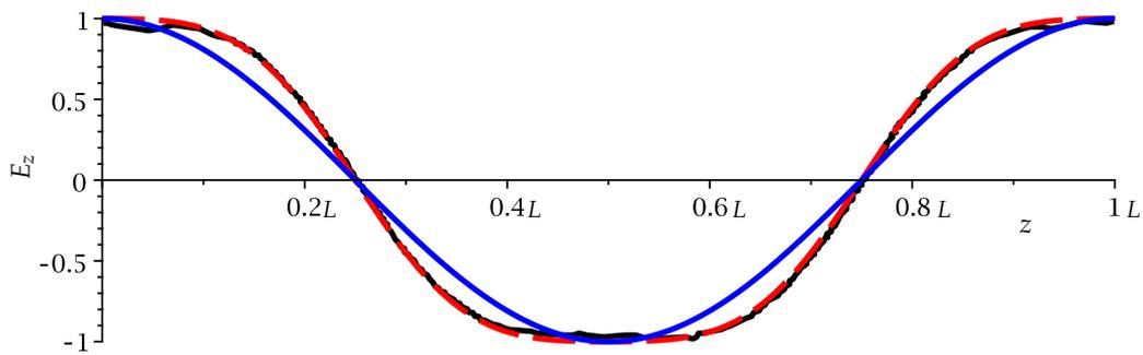
**Figure 9.** Field profile shaping in a metallic waveguide containing a  $4 \times 4$  array of infinitely long wires of varying radii and with  $L = 80.61$  mm. The simulated field profile  $E_z$  itself is normalised and shown with solid black lines, and is compared with the ideal Mathieu function profile shown as a dashed red curve, with a sinusoid shown in blue as a reference. In the simulation, CST gave the maximum longitudinal field as  $3.28 \times 10^7$   $\text{Vm}^{-1}$ .
