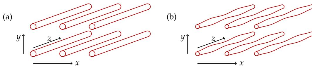
**Figure 1.** A wire medium is formed from an array of parallel metal or dielectric wires. In this work we use results based on rectangular arrays of (a) wires with uniform radii to predict the parameters needed for customised (b) wires with varying radii that generate a desired subwavelength field profile shaping.
