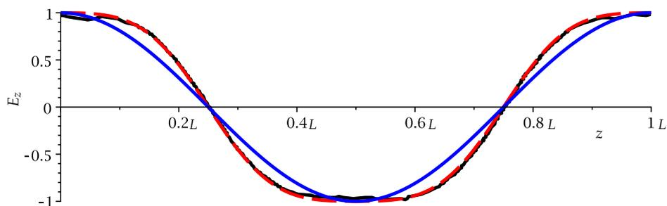
**Figure 13.** Profile of  $E_z$  component for a waveguide with  $2 \times 2$  infinitely long wires of varying radii (solid Black) in comparison with Mathieu function (dashed red) and sin function (blue). Here  $L = 127.4$  mm. Both  $E_z$  and the Mathieu function are normalised. However CST gave the maximum longitudinal field as  $6.03 \times 10^7$   $\text{Vm}^{-1}$ .
