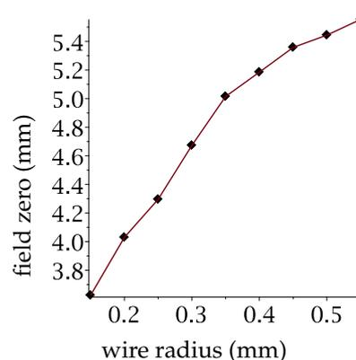
**Figure 4.** How the radius of the wire affects the distance from the wire at which the longitudinal field  $E_z$  passes through zero. This result was calculated using periodic boundary conditions for an infinite rectangular array of uniform and infinitely long wires.
