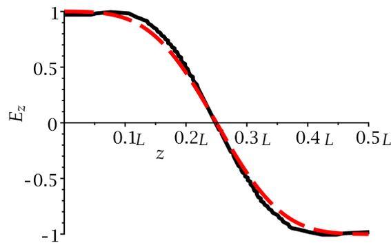
**Figure 11.** Field profile shaping in a metallic waveguide containing a  $4 \times 4$  array of wires with varying radii in a metallic cavity, and with  $L = 80.61$  mm. The simulated field profile  $E_z$  itself is normalised and shown with solid black lines, and is compared with the ideal Mathieu function profile shown as a dashed red curve.
