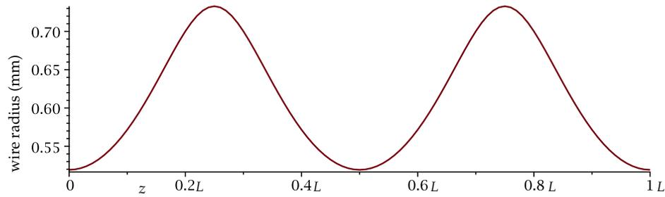
**Figure 7.** By combining our desired field profile (the Mathieu function of (1)) with the plasma frequency response in Figure 6 we can predict the necessary radius variation for our  $4 \times 4$  wire array in a waveguide. The result is shown here, with a radius that changes by about  $\pm 15\%$  around its average value.
