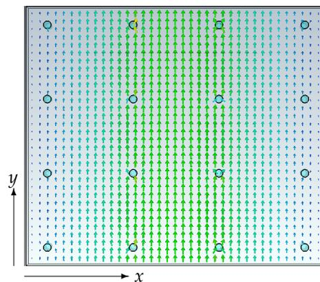
**Figure 14.** An example showing the electric field vectors on a slice in the  $(x, y)$  plane perpendicular to the wires. Most of the field modes near our desired longitudinal modes are of this transverse type, and should not be excited by a carefully designed (longitudinal) excitation field. The dimensions of the waveguide are the same as in Figure 8.
