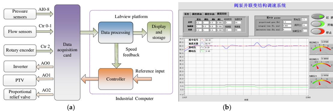
Figure 5. Measurement and control system. (a) Control principle; (b) Interface.
