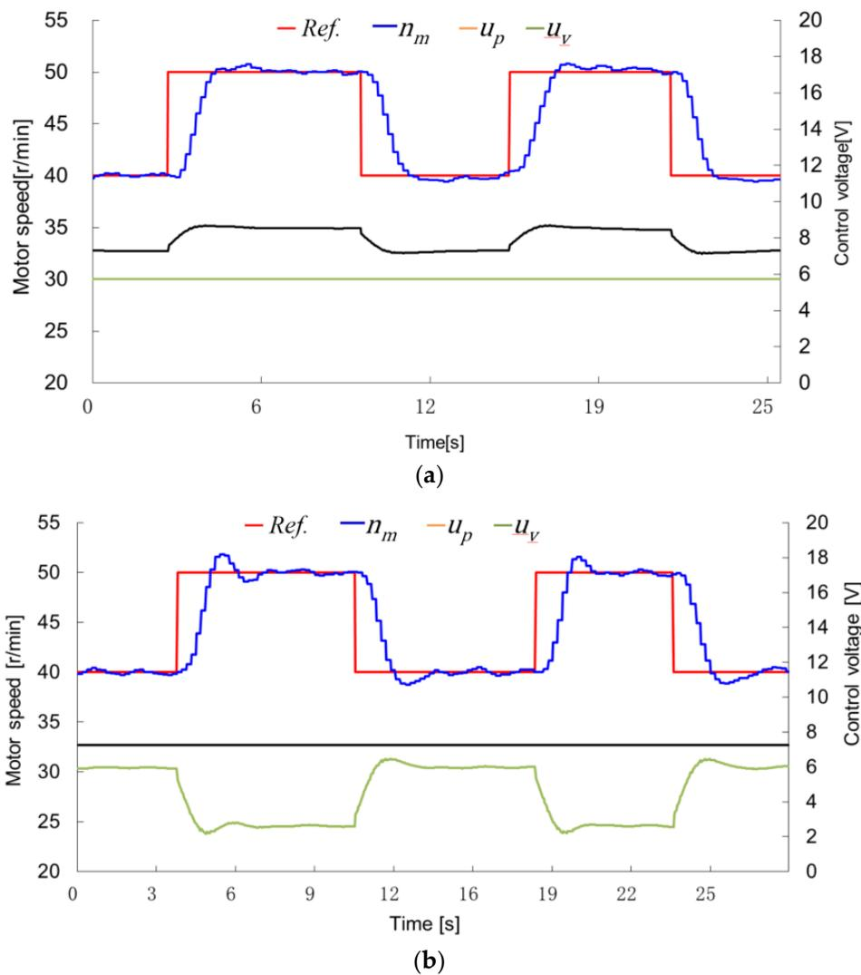
Figure 6. Step response of pump control and valve control. (a) Pump control circuit; (b) Valve control circuit.
