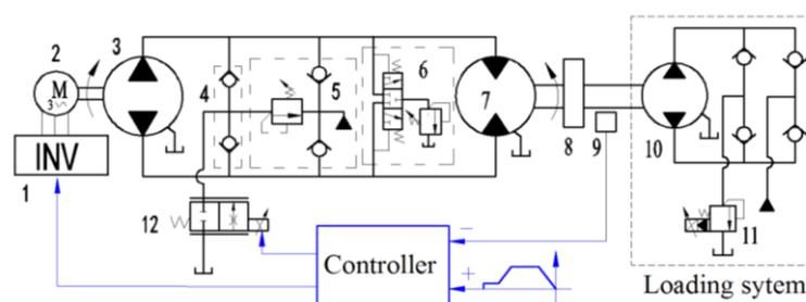
**Figure 1.** Schematic framework of LVPC (leaking valve-pump parallel control) system. 1—Inverter; 2—electric motor; 3—Fixed displacement pump; 4—Shuttle valve; 5—Oil replenishing device; 6—Flushing device; 7—Hydraulic motor; 8—Inertia; 9—Encoder; 10—Loading pump; 11—Proportional relief valve; 12—PTV (proportional throttle valve).
