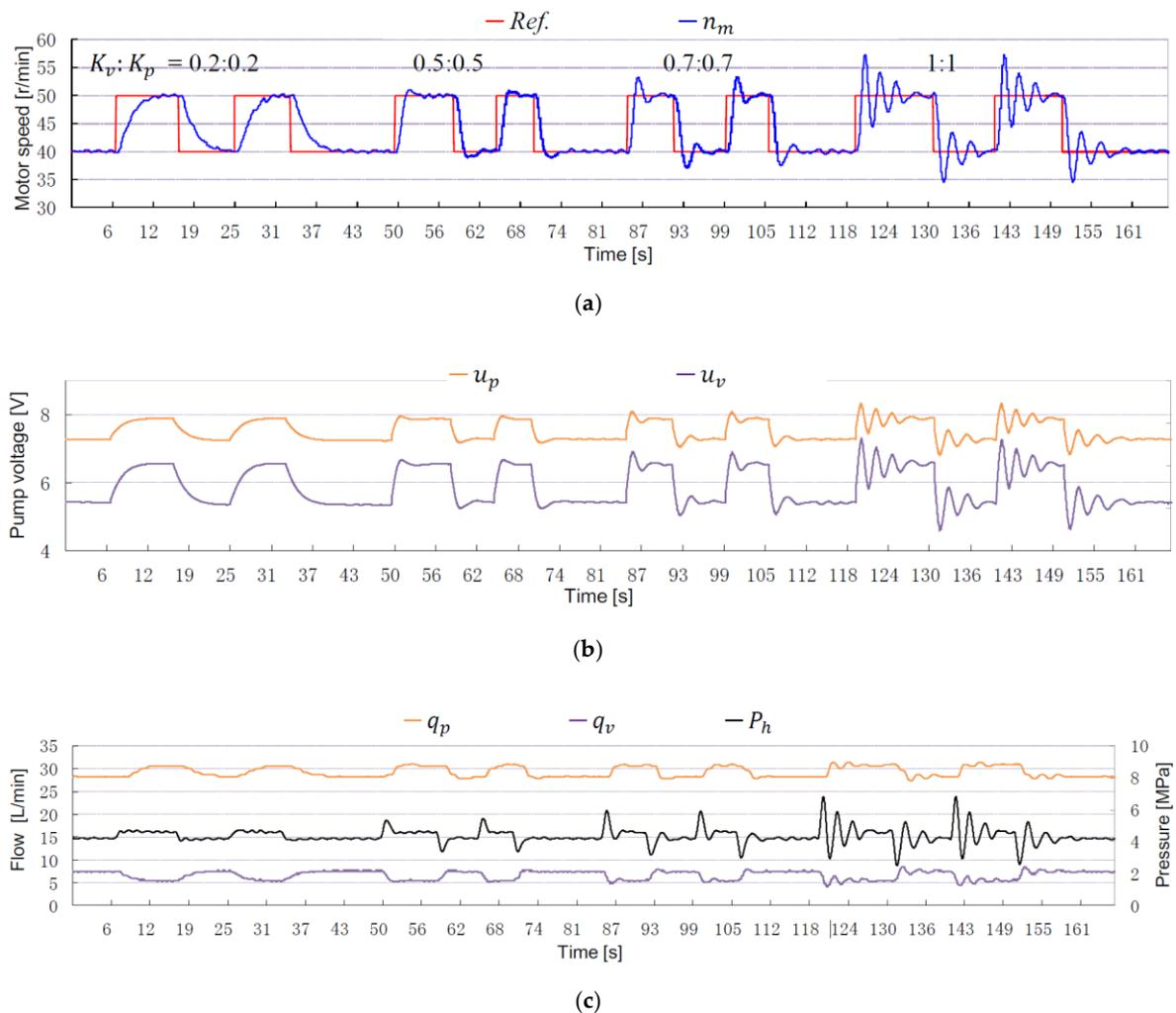
**Figure 8.** Step response to reference inputs when  $K_{vp} = 1$ . (a) Motor speed response; (b) Pump and valve voltage variation; (c) System pressure and flow response.
