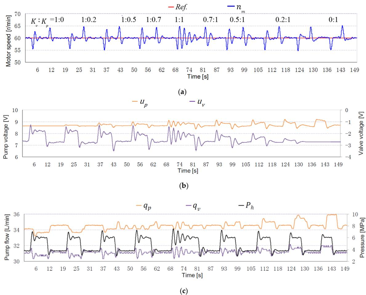
**Figure 9.** Step response to loads under different weight ratios  $K_{vp}$ . (a) Motor speed response; (b) Pump and valve voltage variation; (c) System pressure and flow response.
