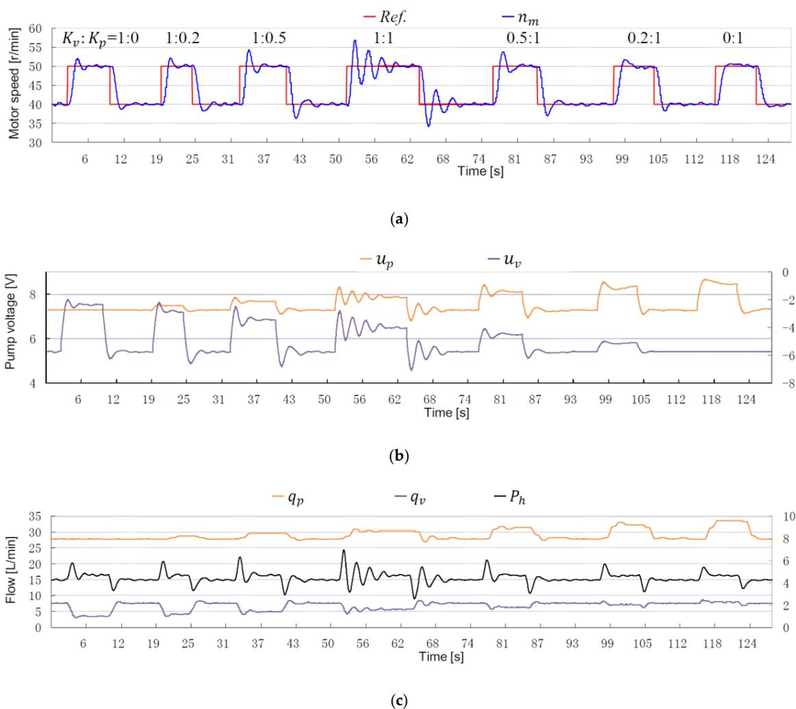
**Figure 7.** Step response to reference inputs under different weight ratios  $K_{vp}$ . (a) Motor speed response; (b) Pump and valve voltage variation; (c) System pressure and flow response.
