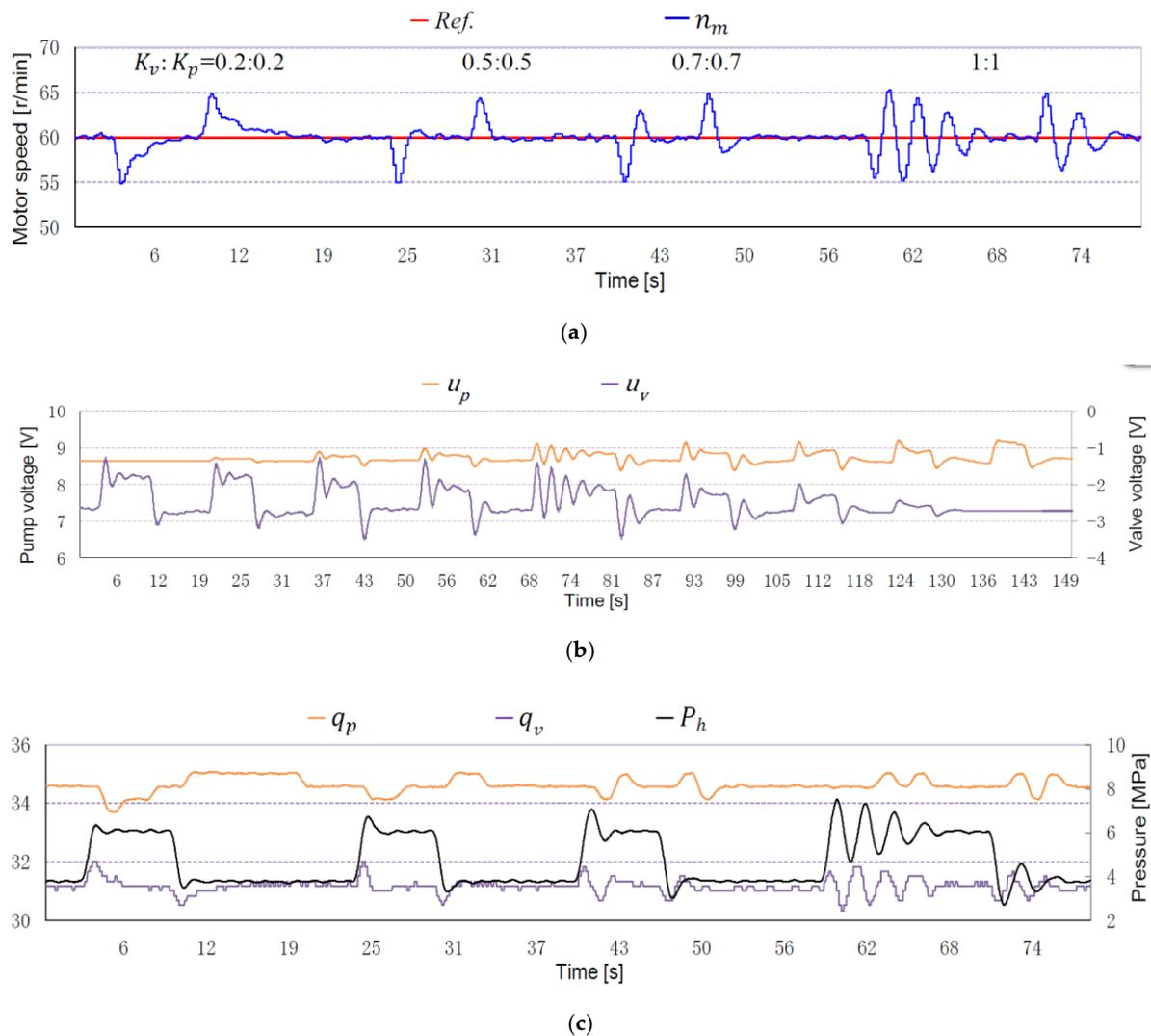
**Figure 10.** Step response to loads when  $K_{vp} = 1$ . (a) Motor speed response; (b) Pump and valve voltage variation; (c) System pressure and flow response.
