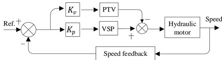
Figure 2. Control principle of leaking valve-pump parallel control.
