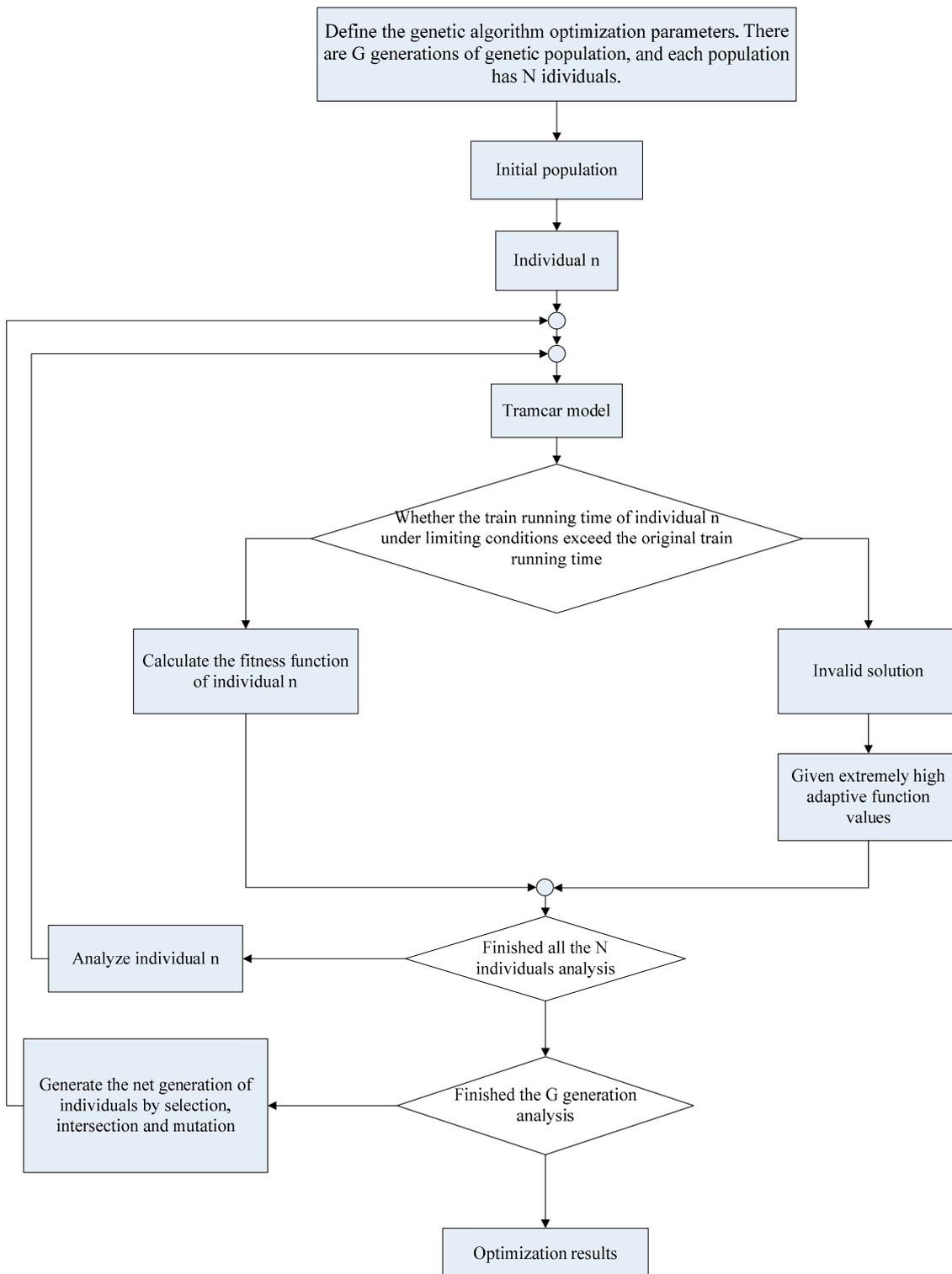
Figure 12. Optimization of the energy management strategy using a genetic algorithm.
