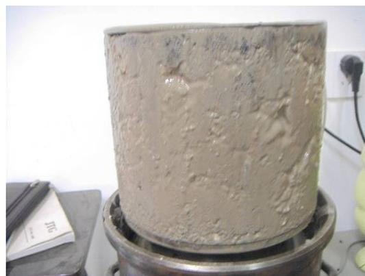
Figure 11. Specimen appearance under gyration compaction.
