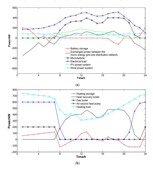
**Figure 12.** Electrical load (**a**) and heating load (**b**) dispatching schemes of the micro energy grid for a typical day in the winter when the distribution network comprising the micro energy grid was in the optimal dispatching state.
