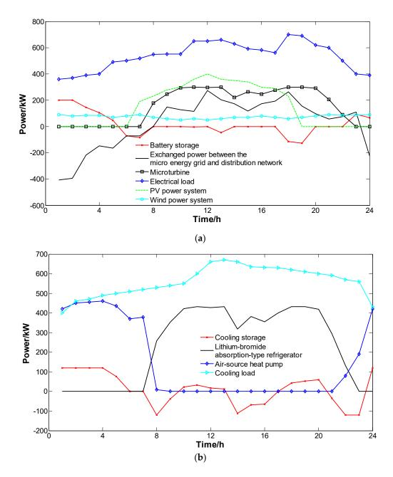
**Figure 13.** Electrical load (**a**) and cooling load (**b**) dispatching schemes of the micro energy grid for a typical day in the summer when the distribution network comprising the micro energy grid was in the optimal dispatching state.
