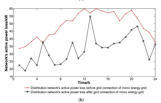
**Figure 9.** Comparison of the network's active power loss before and after the grid connection of the micro energy grid on a typical day in the winter (**a**), and in the summer (**b**).
