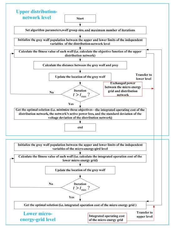
**Figure 4.** Flow chart of the bi-level optimal model of the distribution network comprising the micro energy grid, based on the improved GWO algorithm.
