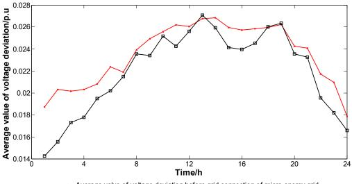
Average value of voltage deviation before grid connection of micro energy grid Average value of voltage deviation after grid connection of micro energy grid
