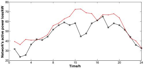
Distribution network's active power loss before grid connection of micro energy grid
