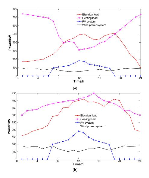
**Figure 8.** Cooling, heating, and electrical load curves, and wind power and photovoltaic (PV) prediction curves for the micro-energy grid on a typical day in the winter (**a**), and in the summer (**b**).
