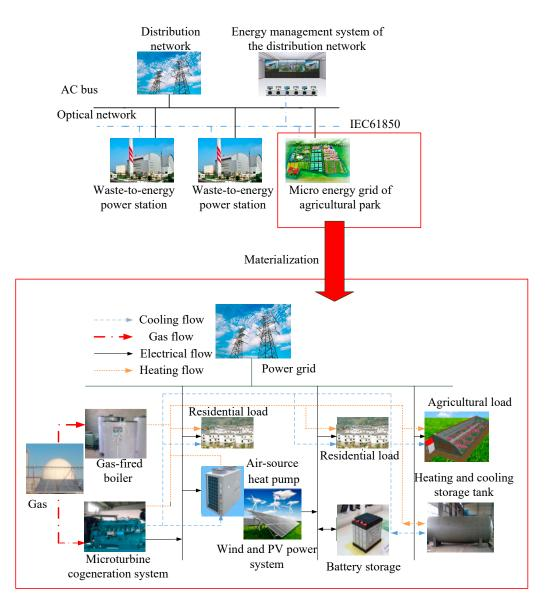
Figure 2. Operating structure of a distribution network comprising a micro energy grid.
