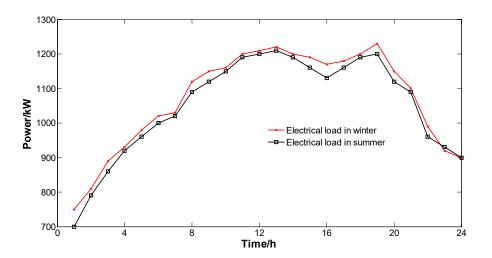
**Figure 7.** Electrical load curve of the distribution network on a typical day in the winter and in the summer.
