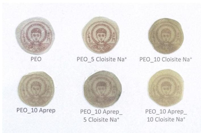
**Figure 2.** Transparency of films made of pure PEO, drug-loaded (10 wt %) PEO (PEO\_10Aprep), nanocomposites (5 and 10 wt % clay, PEO\_5Cloisite-Na<sup>+</sup> and PEO\_10Cloisite-Na<sup>+</sup>, respectively) and drug-loaded nanocomposites (PEO\_10Aprep\_5Cloisite-Na<sup>+</sup>, PEO\_10Aprep\_10Cloisite-Na<sup>+</sup>, respectively).
