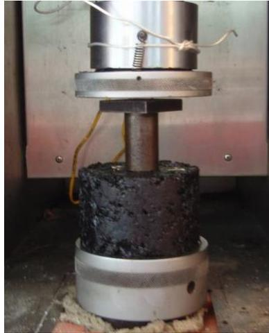
**Figure 4.** Uniaxial penetration test.
