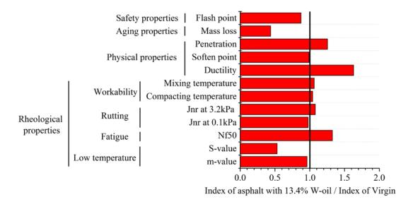
Figure 21. Ratio of Index of Virgin Asphalt and Rejuvenated Asphalt with 13.4% W-oil.
