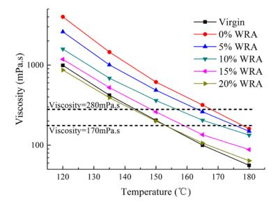
Figure 14. Viscosity-Temperature Curve of Virgin, Aged, and Rejuvenated Asphalt.
