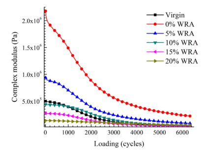
Figure 18. Change of Complex Modulus under Loading.
