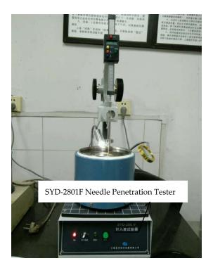
Figure 6. The Needle Penetration Tester.
