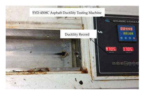
Figure 8. The Ductility Testing Machine.
