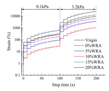
Figure 16. Multiple Stress Creep Recovery (MSCR) Curve of Virgin, Aged, and Rejuvenated Asphalt.
