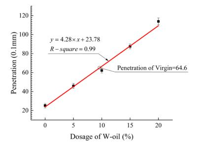
Figure 11. Penetration of Virgin, Aged, and Rejuvenated Asphalt.
