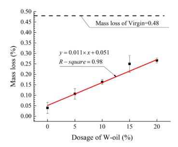
Figure 10. Mass Loss of Virgin, Aged, and Rejuvenated Asphalt.
