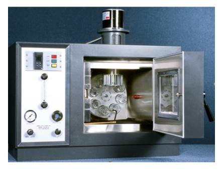
Figure 5. The Rolling Thin Film Oven.
