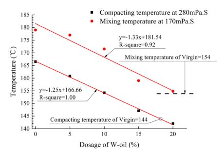
Figure 15. Mixing and Compacting Temperature of Virgin, Aged, and Rejuvenated Asphalt.
