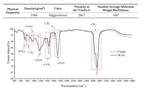
Figure 3. Fourier transform infrared (FTIR) Spectra of W-oil and Virgin Asphalt.
