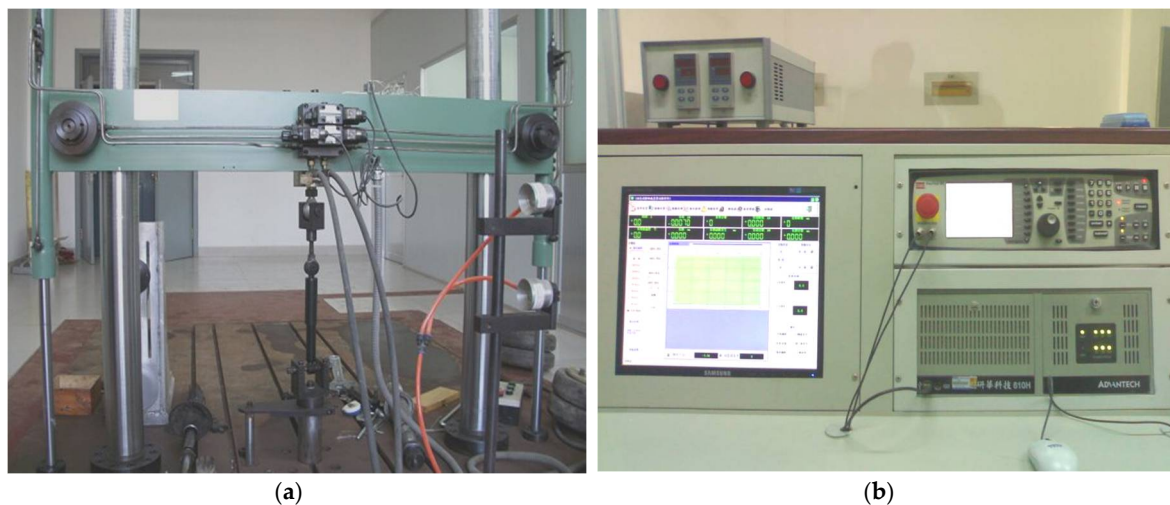
Figure 7. Damper test: (a) the test bench; and (b) the master computer.
