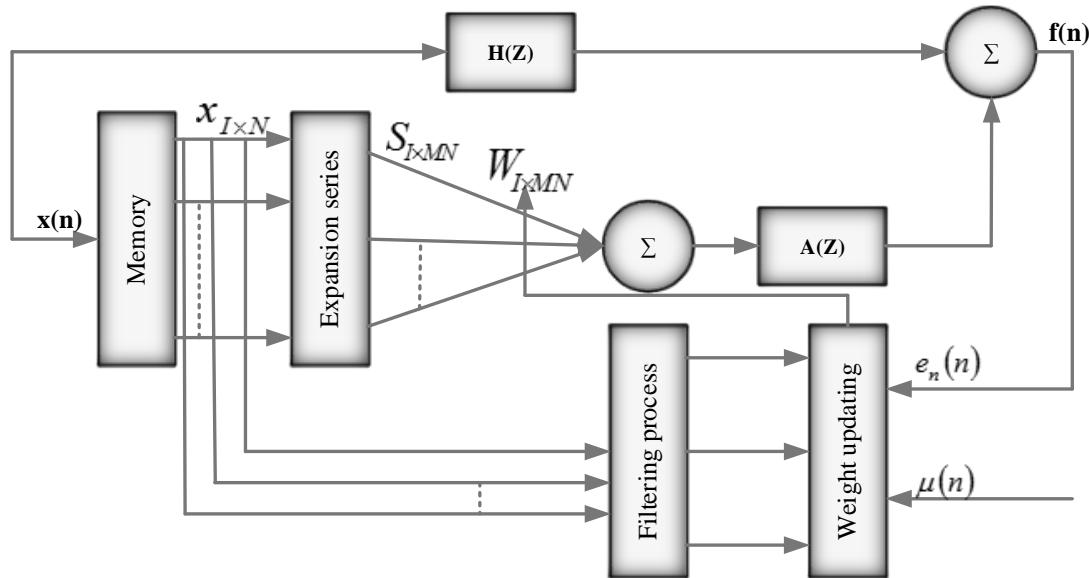
**Figure 2.** Active noise control with modified FsLMS.
