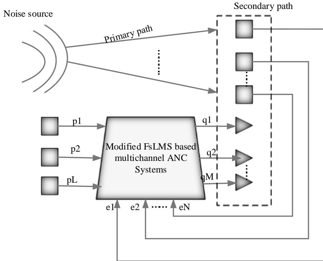
**Figure 1.** Schematic of MFsLMS based on multichannel ANC.
