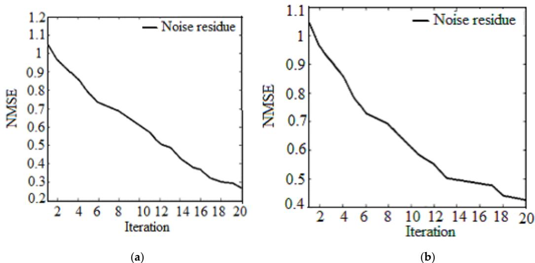
**Figure 8.** Number of iterations versus normalized mean square error (a) Proposed method; (b) Existing method (FsLMS).
