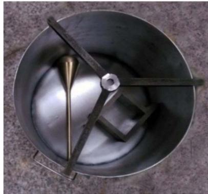
**Figure 3.** Apparatus for Lueer test.
