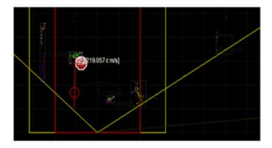
**Figure 9.** There is an object in the danger zone and collision is highly probable. A stop sign appears on the screen, an alarm signal plays and automatic brakes are activated. Heading of the object can be seen with a red line and possible collision position can be seen with the red circle.
