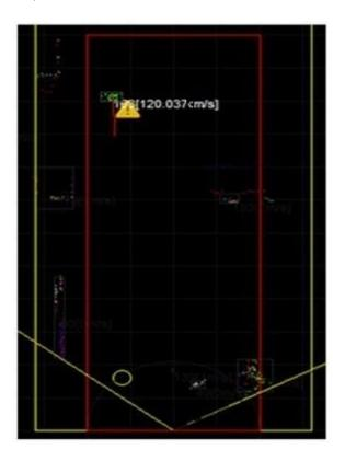
**Figure 8.** There is an object in danger zone and getting closer to tram slowly. An exclamation mark appears on the screen and an alarm signal is activated. Heading of moving object can be seen with a red line and possible collision position can be seen as a yellow circle on the Figure 8.
