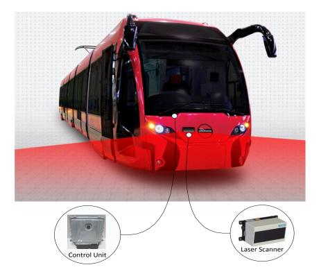
**Figure 1.** Ladar Digital-Multilayer Range Scanner (LD-MRS) laser scanner mounted in front of the test vehicle named "Silkworm" which is manufactured by Durmazlar Machine Inc. and control unit of the test vehicle.
