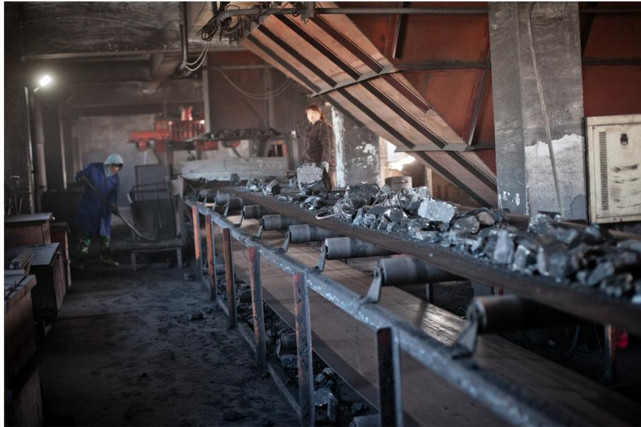
**Figure 1.** Manual separation of coal and gangue.
