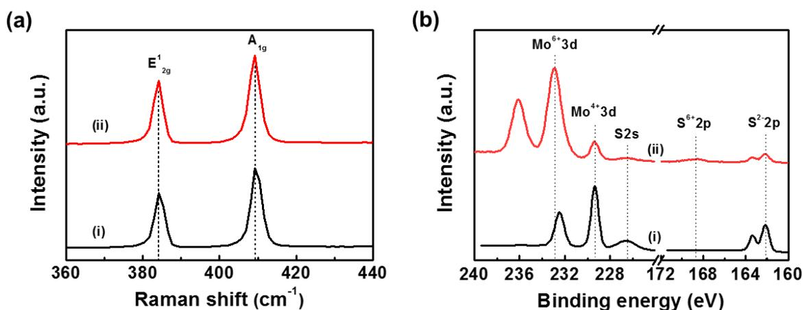
**Figure S2.** (a) Raman and (b) XPS spectra of (i) pristine and (ii) UV-ozone treated MoS<sub>2</sub>.
