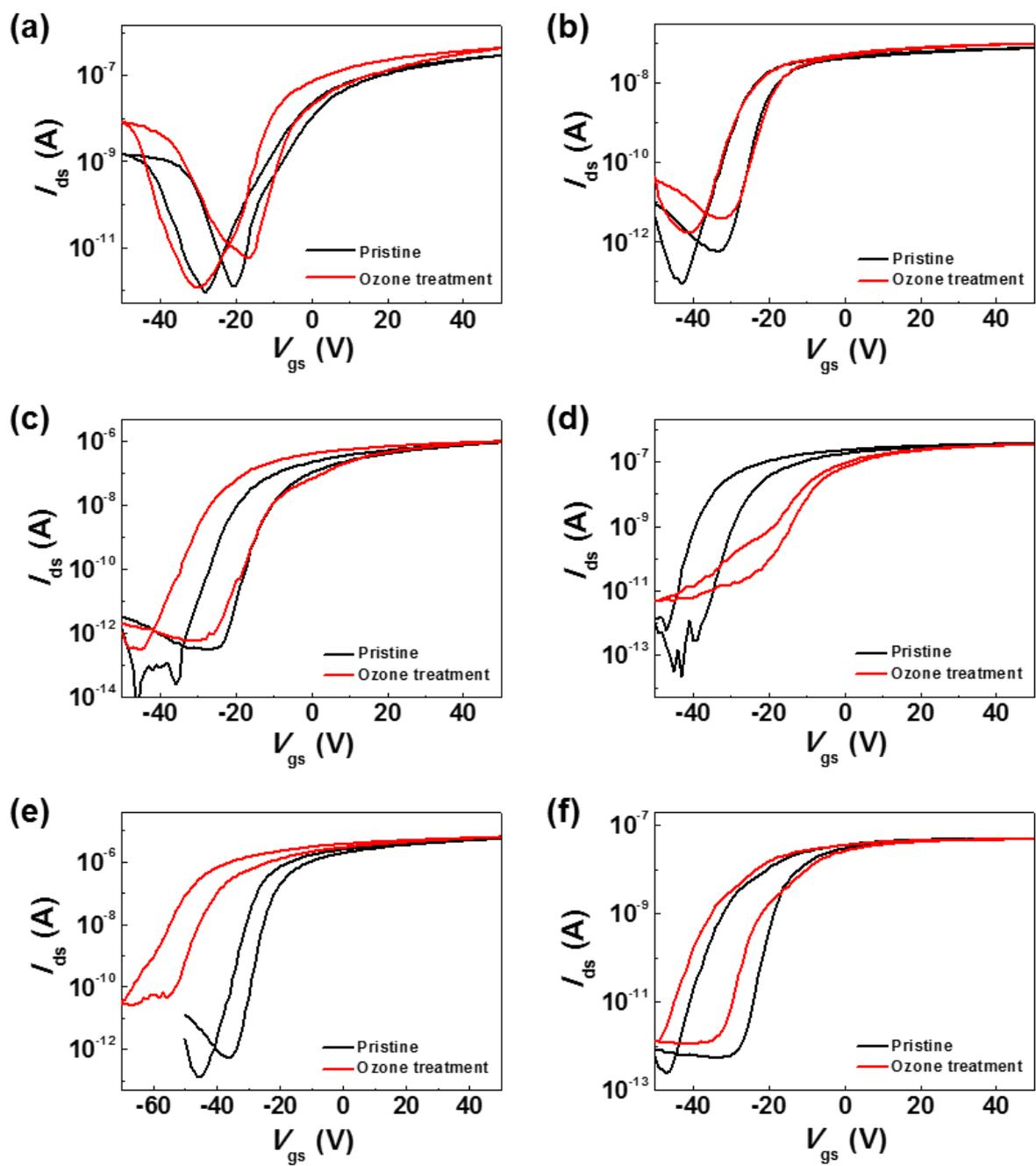
**Figure S4.** Transfer characteristics of six MoS<sub>2</sub> TFTs without Al<sub>2</sub>O<sub>3</sub> passivation before (i.e., pristine) and after UV-ozone treatment.
