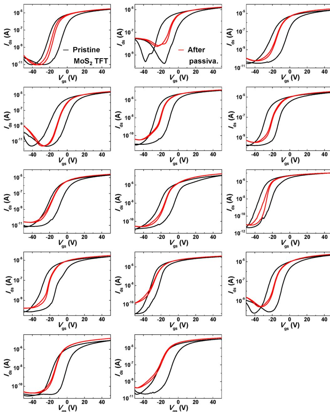
**Figure S3.** Transfer characteristics of 14 MoS<sub>2</sub> TFTs before (black line) and after (red line) Al<sub>2</sub>O<sub>3</sub> passivation.
