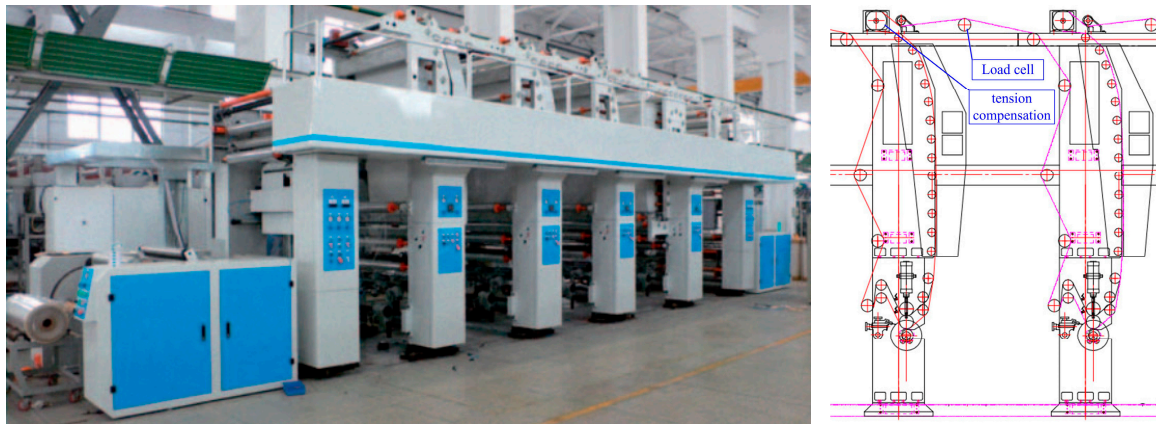
Figure 3. Gravure printed electronics experimental setup.
