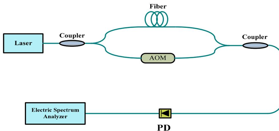
Figure 2. The diagram of the linewidth measurement system.
