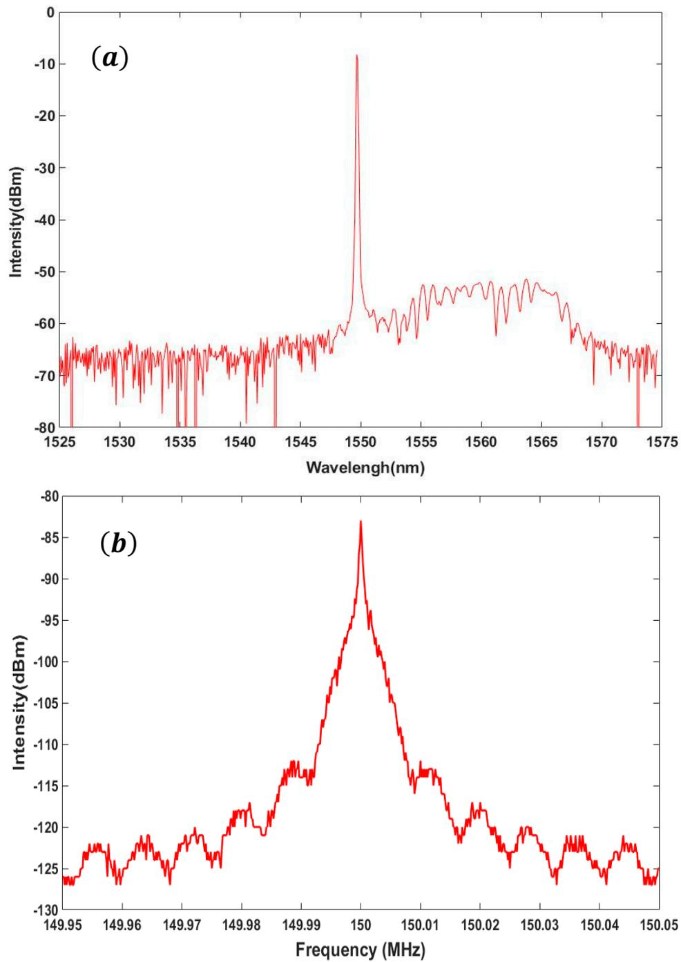
**Figure 6.** Output spectrum and power spectrum of 25 km delayed self-heterodyne of 20 W laser signal. (a) Shows the output spectrum of the power amplifier at the maximum output power. (b) Shows the actual recorded power spectrum at the maximum output power of laser measured with 25 km delayed fiber.
