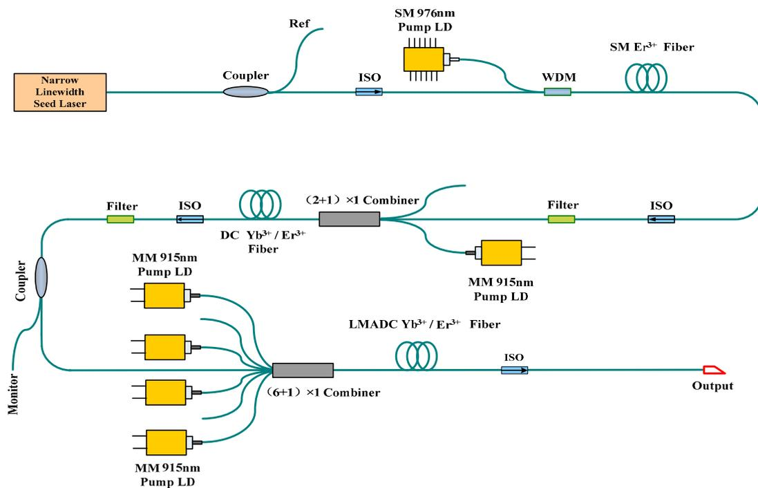
Figure 1. Schematic diagram of the experimental setup for the  $\text{Er}^{3+}:\text{Yb}^{3+}$ -co-doped fiber amplifier (EYDFA) system.
