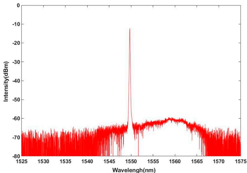
Figure 4. Output spectrum of the second preamplifier.
