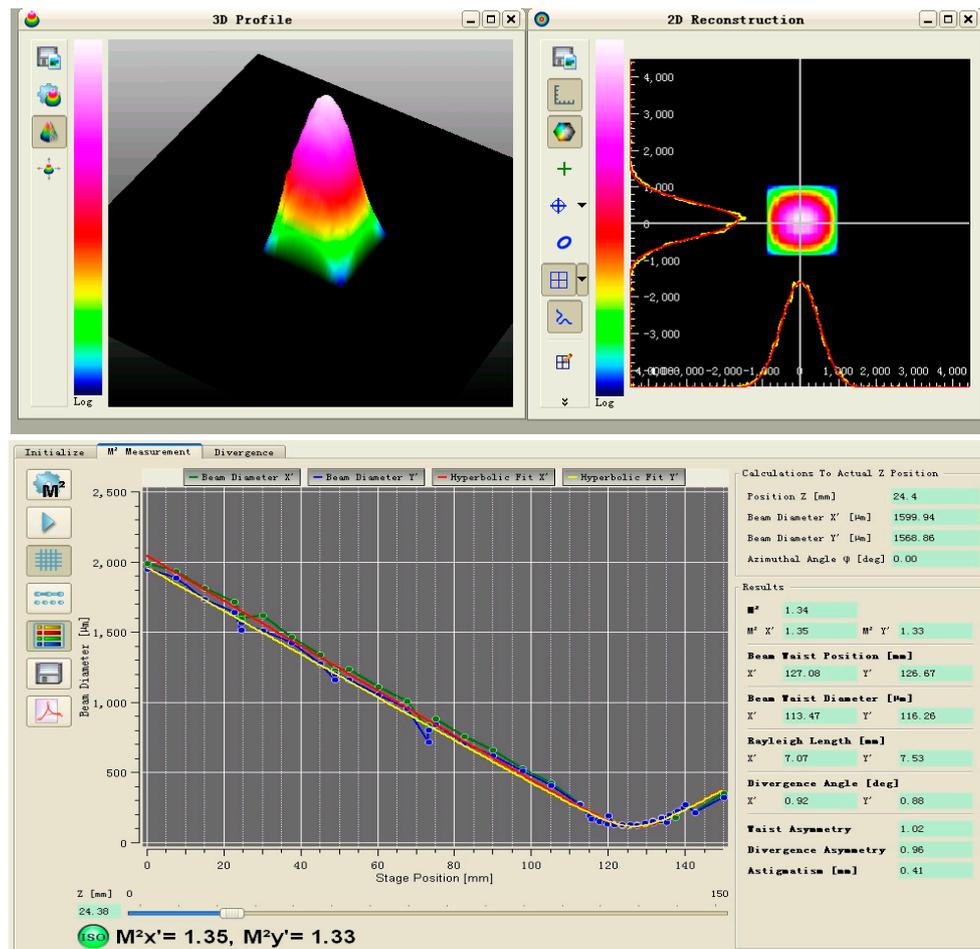
Figure 9. Beam quality  $M^2$  measurement results.
