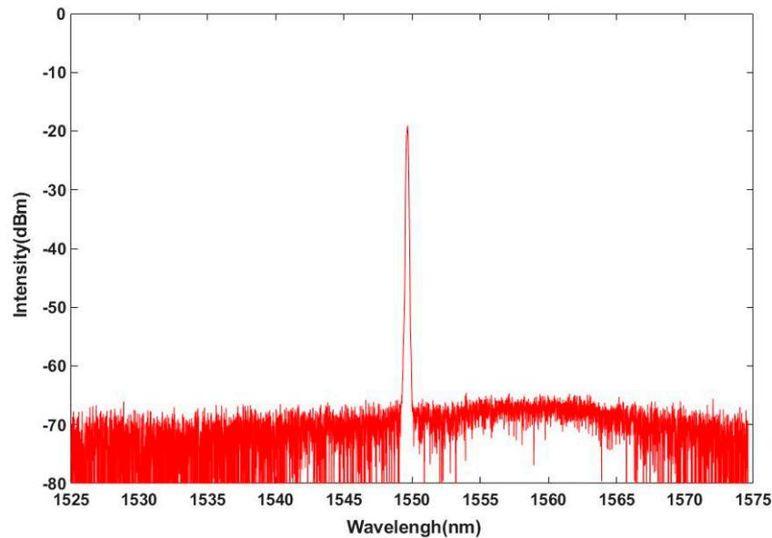
Figure 3. Output spectrum of the seed signal.
