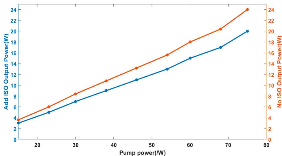
Figure 5. Output power of the last pump amplifier versus pump power.
