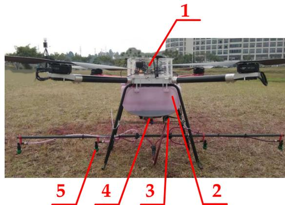
**Figure 6.** Physical diagram of the variable spraying system. **Note:** 1. Prescription map interpretation system and spray controller; 2. medicine case; 3. Hall flow sensor; 4. miniature diaphragm pump; 5. pressure nozzle.
