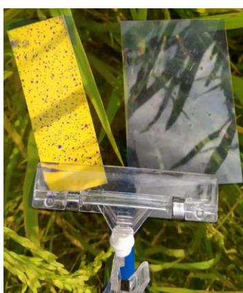
**Figure 17.** Layout of the Mylar card and water-sensitive paper.
