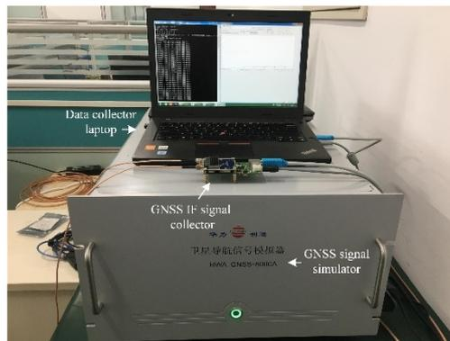
Figure 3. Data collection process with GNSS hardware simulator.
