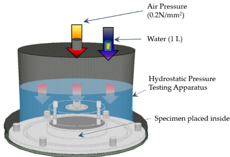
**Figure 10.** Hydrostatic pressure testing illustration.
