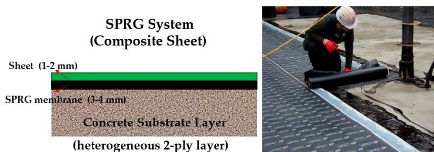
**Figure 2.** Separate and integrated 2-ply type SPRG waterproofing systems.
