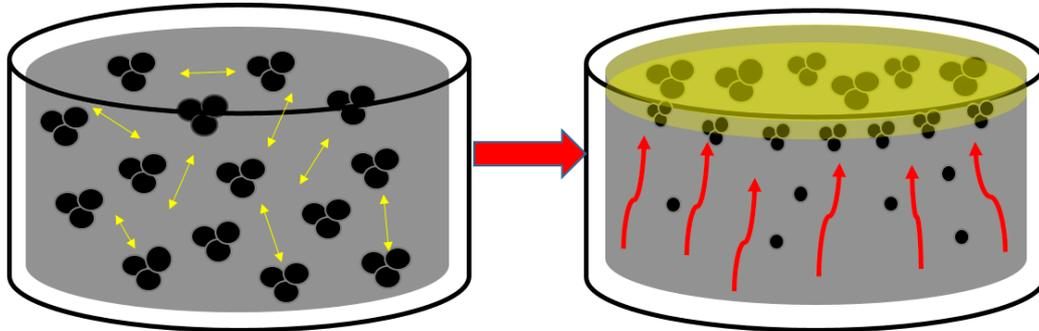
**Figure 5.** Property changes in SPRG following the screw-mixing process; facilitated emulsion breaking following filler particle and globule dispersion due to screw mixing.
