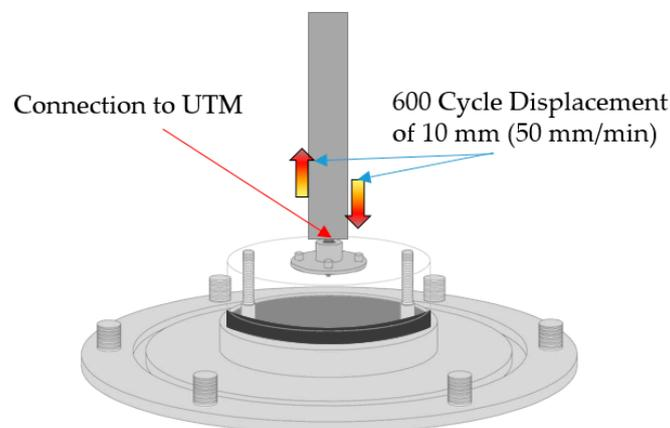
**Figure 11.** Illustration of substrate movement resistance testing.
