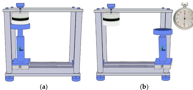
**Figure 9.** Test method for adhesion on wet substrate; (a) specimen placement; (b) water flow testing.
