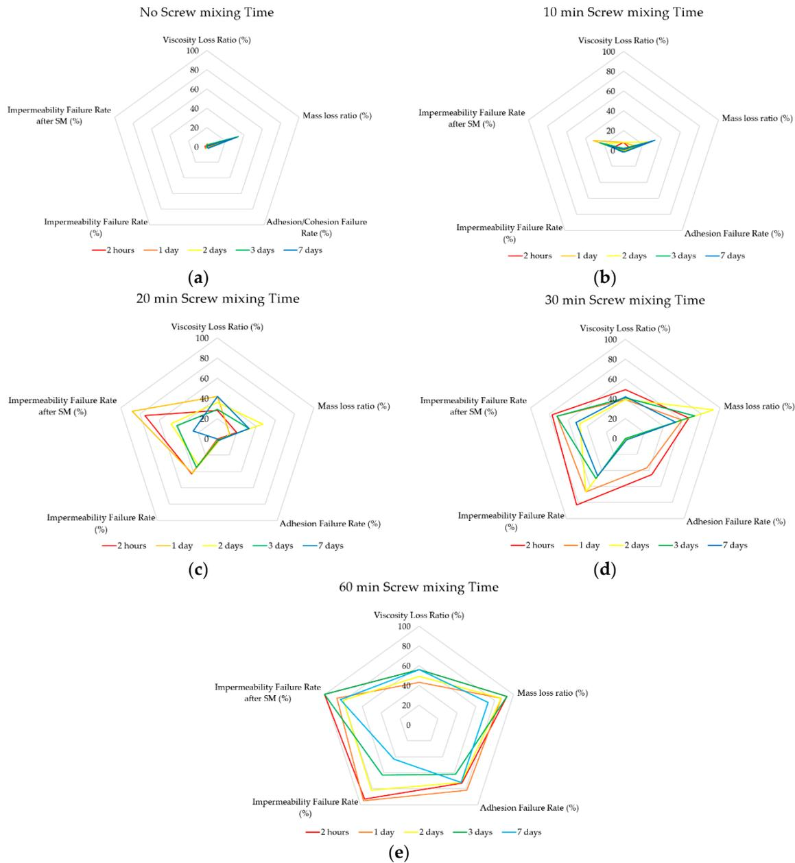
**Figure 13.** Radar charts for comparative evaluation of overall waterproofing performance; (a) results for no screw mixing; (b) results for 10 min of screw mixing; (c) results for 20 min of screw mixing; (d) results for 30 min of screw mixing; (e) results for 60 min of screw mixing.
