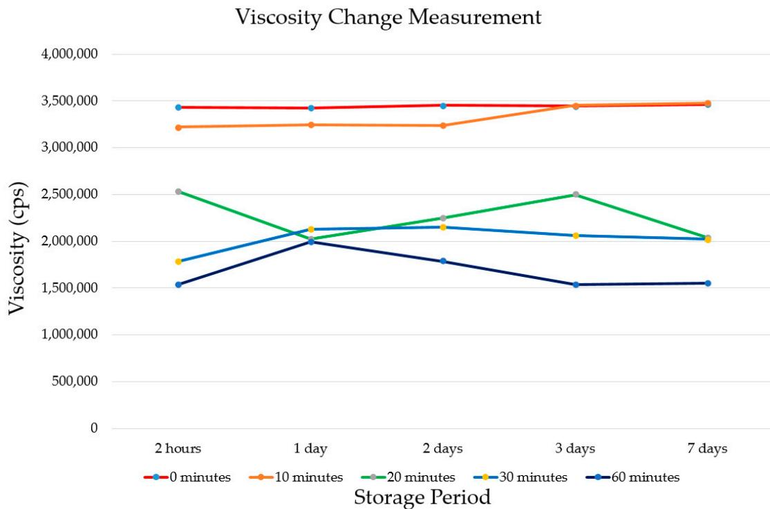
**Figure 12.** SPRG viscosity change over different storage periods based on respective screw-mixing time.
