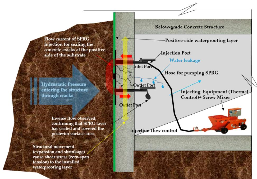
**Figure 1.** Common Synthetic polymerized rubber gel injection in a below-grade concrete structure.
