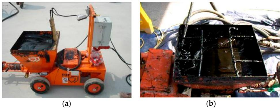
Figure 3. SPRG Gel screw-mixing process prior to application; (a) screw mixing SPRG; (b) reduced viscosity after mixing.
