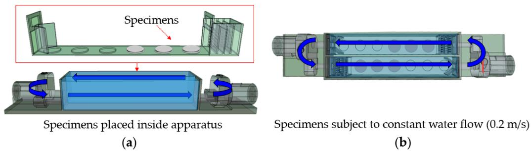
**Figure 8.** Test method apparatus; (a) specimen placement; (b) water flow testing.
