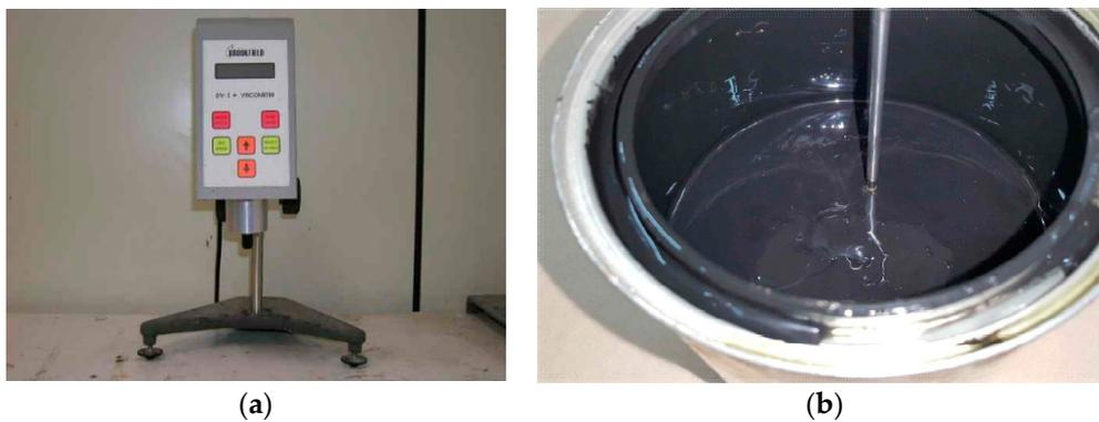
**Figure 7.** Brookfield viscometer; (a) apparatus; (b) measuring SPRG viscosity.
