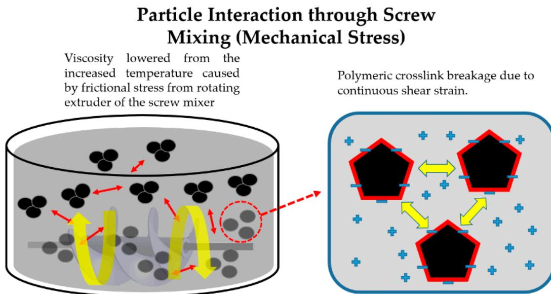
**Figure 4.** Polymeric degradation due to continuous shear strain of screw-mixing process.
