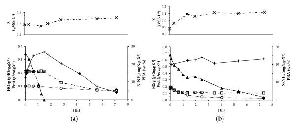
**Figure 2.** Typical profiles of biomass concentration  $(X, \times)$ , specific concentrations of organic acids (*H.Org*,  $\blacktriangle$ ), proteins (*Prot*,  $\bigcirc$ ) and ammonia–nitrogen (*N-NH*<sub>3</sub>,  $\Box$ ), and biomass PHA content (*PHA*, +) obtained in SBR's cycles in Period I (**a**) and Period IV (**b**).
