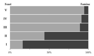
**Figure 6.** Average fractions of ammonia–nitrogen (N–NH<sub>3</sub>) consumption in the feast (light grey) and famine (dark grey) phases of the selected SBR, during the five different operational periods (I–V). The consumption percentages are based on the total consumed ammonia–nitrogen, during the entire cycle.
