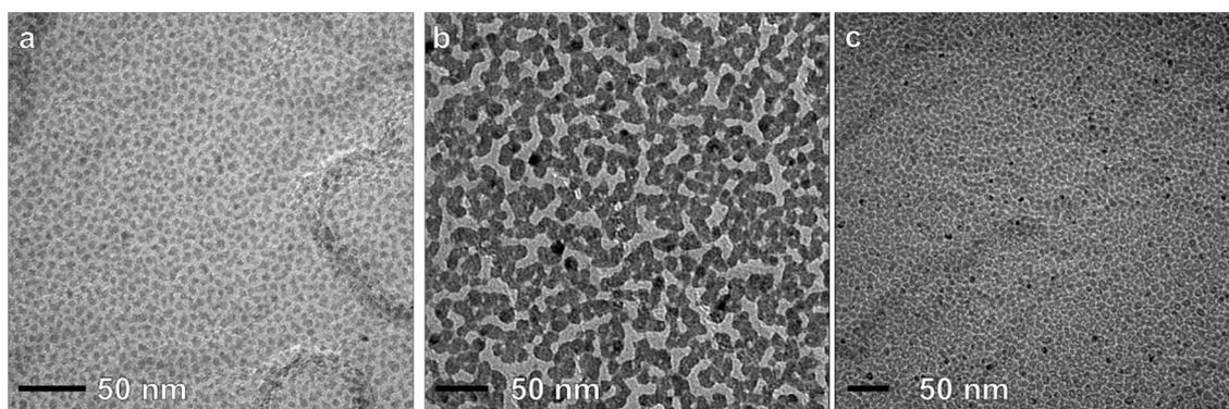
**Figure 1.** Transmission electron microscopy (TEM) micrographs of ZnO-CF<sub>x</sub> nanocomposites having an inorganic phase volume fraction of  $\phi = 0.05$  (a);  $\phi = 0.10$  (b); and  $\phi = 0.15$  (c).
