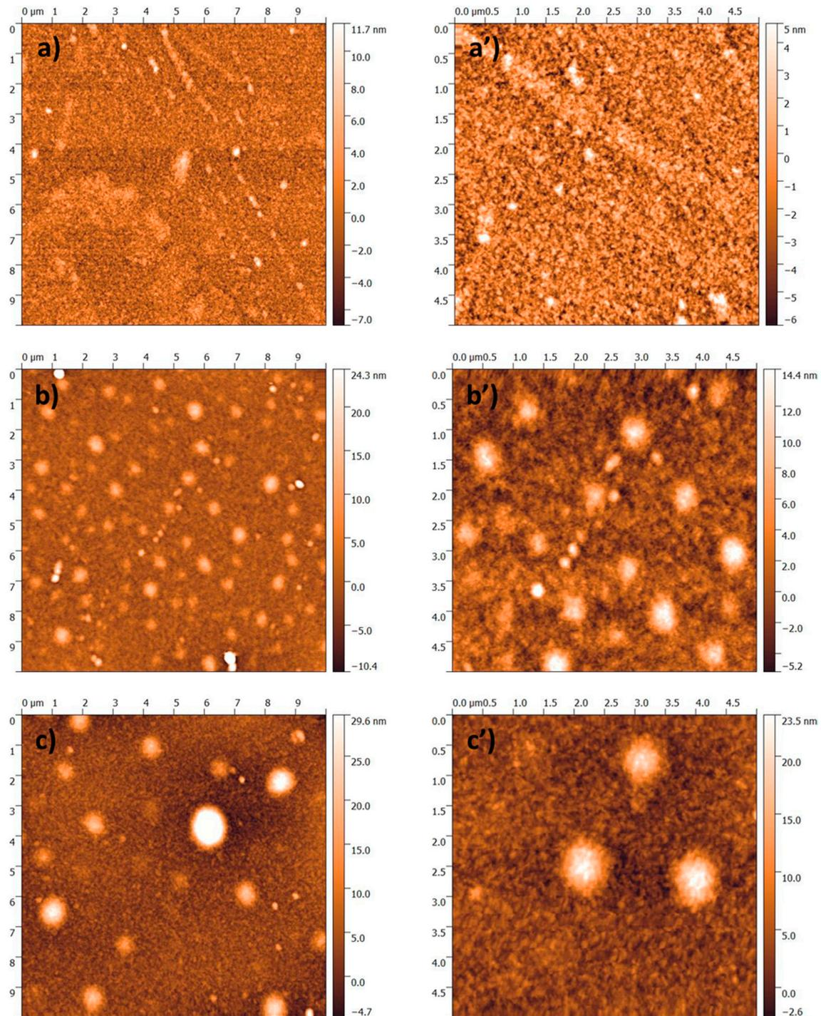
**Figure 2.** Atomic force microscopy (AFM) micrographs of ZnO-CF<sub>x</sub> nanocomposites having an inorganic phase volume fraction of  $\phi = 0.05$  (a–a'),  $\phi = 0.10$  (b–b'), and  $\phi = 0.15$  (c–c').
