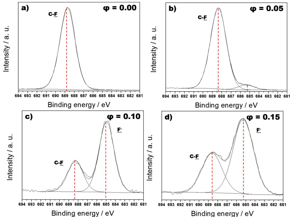
**Figure 3.** F1s XP-high resolution regions of ZnO-CF<sub>x</sub> nanocomposites having an inorganic phase volume fraction  $\phi = 0$  (a),  $\phi = 0.05$  (b),  $\phi = 0.10$  (c), and  $\phi = 0.15$  (d).
