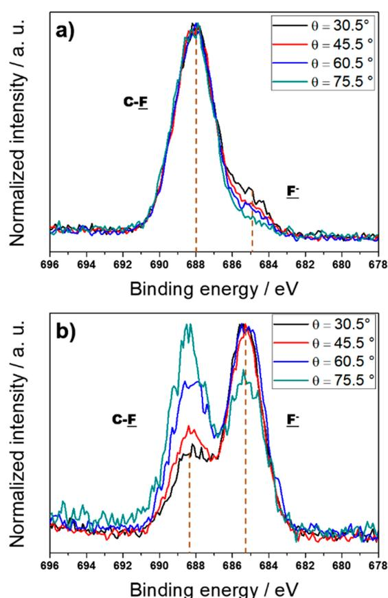
**Figure 5.** F1s XP-high resolution regions of ZnO-CF<sub>x</sub> nanocomposites having an inorganic phase volume fraction of  $\phi = 0.15$  as a function of  $\theta$  and subject to thermal treatment in an oxygenated atmosphere (a) or deposited with an auxiliary O<sub>2</sub> flow (b).
