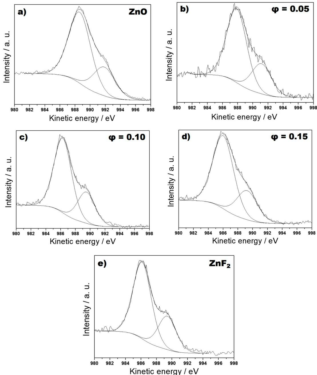
**Figure 4.**  $ZnL_3M_{45}M_{45}$  XP-high resolution regions of  $ZnO-CF_x$  nanocomposites having an inorganic phase volume fraction of  $\phi = 0.05$  (b);  $\phi = 0.10$  (c); and  $\phi = 0.15$  (d). The same region for a pure ZnO film (a) and a  $ZnF_2$  standard (e) is also reported, for comparison.
