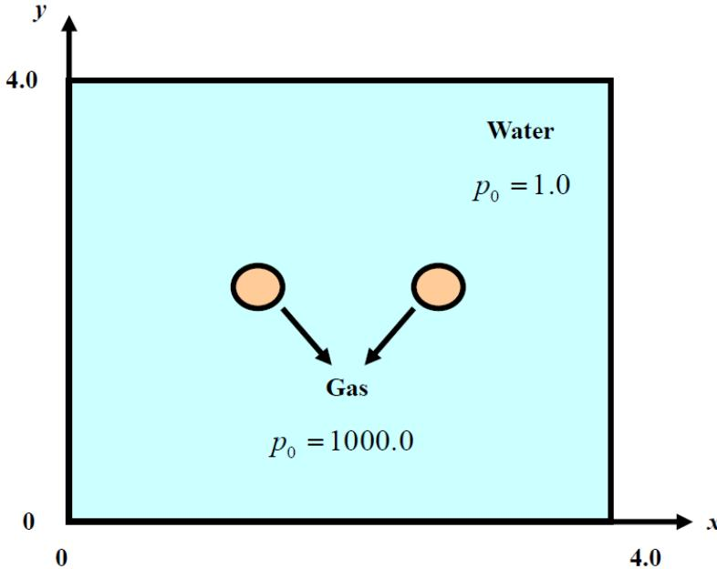
**Figure S3.** The initial configuration of the 2-D double underwater explosion simulation, taken after [2].
