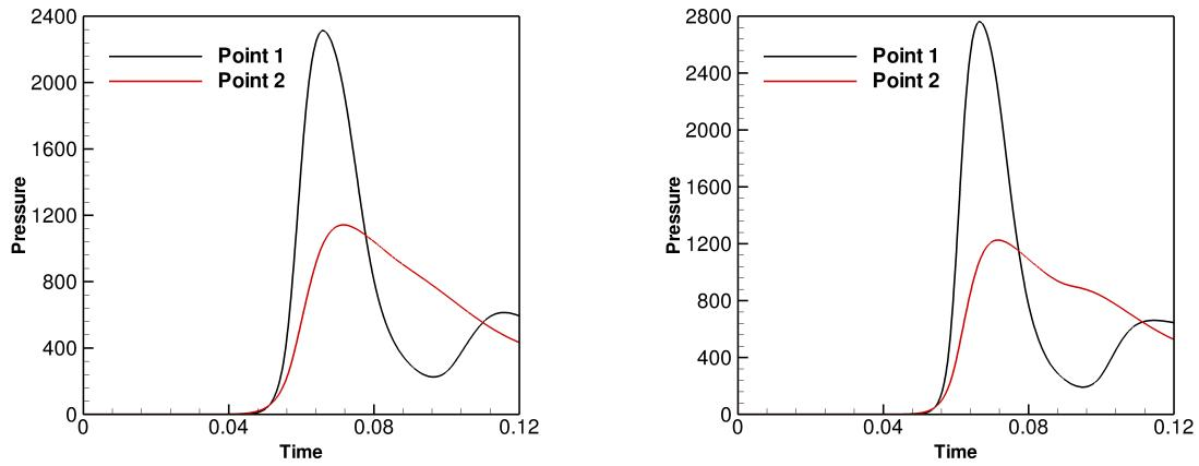
**Figure S6.** The pressure history recorded at the boundaries of the computational domain for an initially bullet-like bubble (Scenario 4); mesh size: (left)  $61 \times 61 \times 61$ ; (right)  $81 \times 81 \times 81$ .
