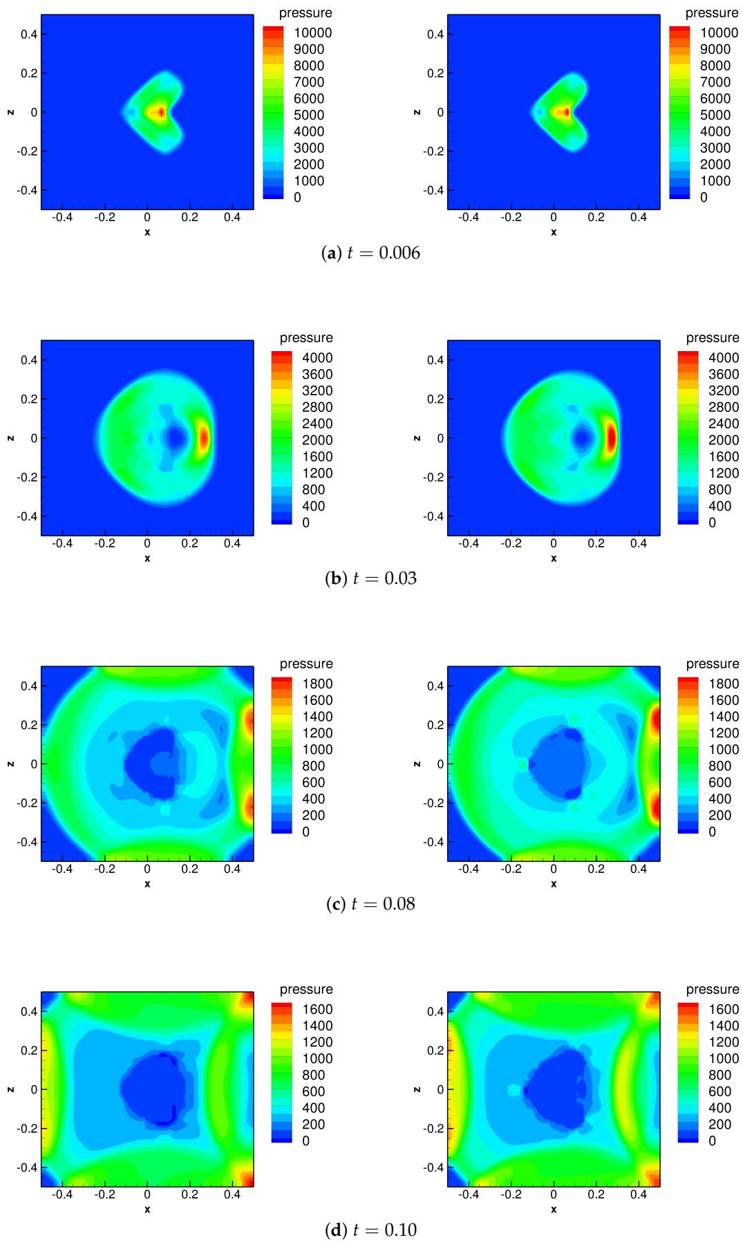
**Figure S5.** The temporal evolution of the pressure field for an initially bullet-like bubble in slice plots ( $y = 0$ ) (Scenario 4); mesh size: (left)  $61 \times 61 \times 61$ ; (right)  $81 \times 81 \times 81$ .
