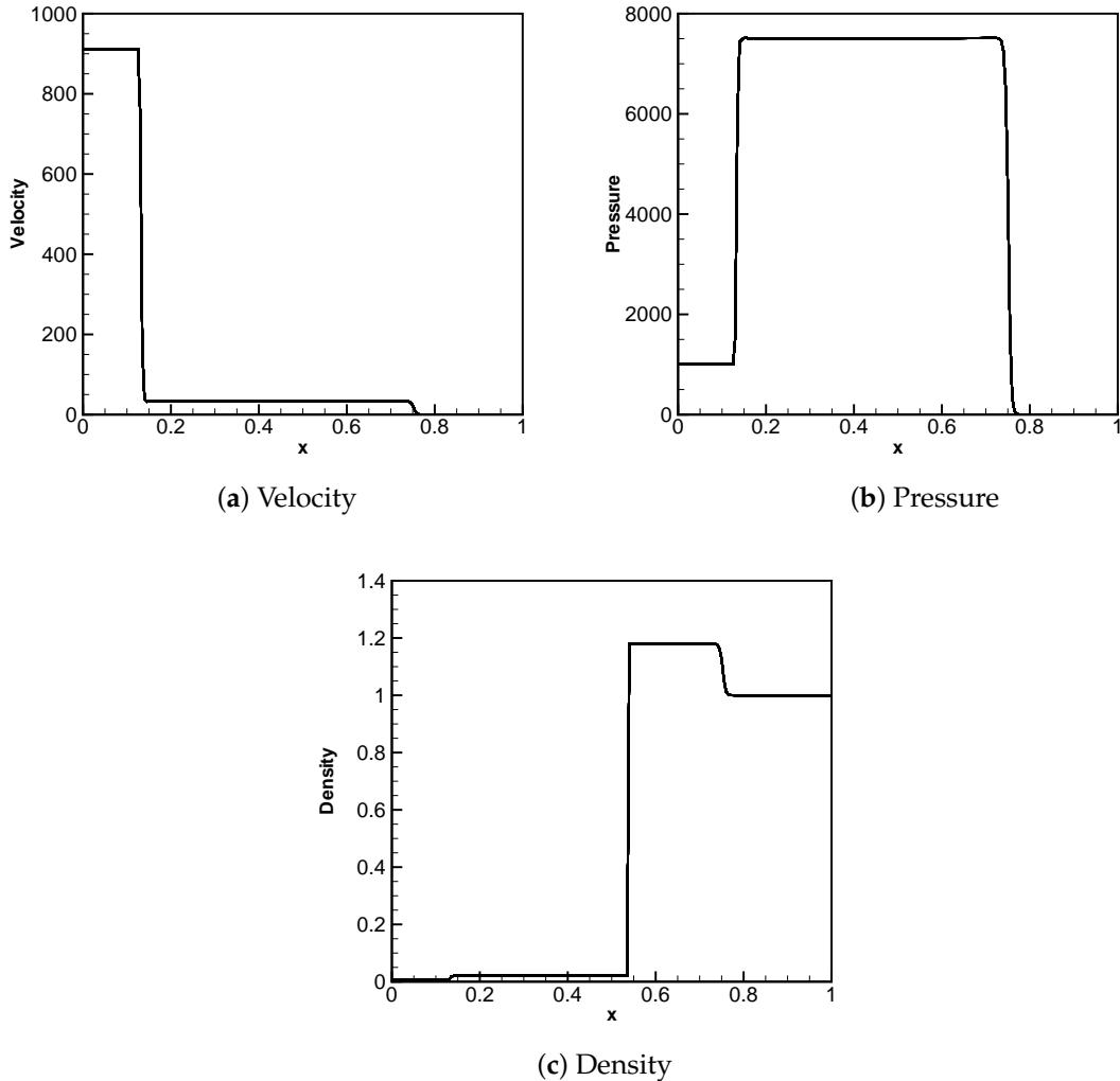
**Figure S2.** The distribution of velocity, pressure and density along  $x$  direction after 350 time steps of computations by using the present 3-D model.
