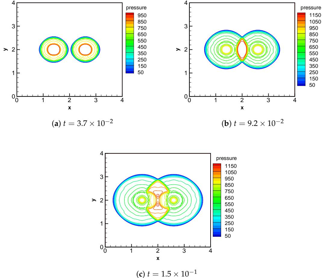
**Figure S4.** The evolutions of the pressure field of the 2-D validation case at different time points by using the 3-D model.
