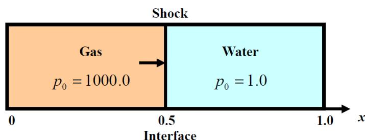
**Figure S1.** The initial setup of the 1-D simulation of the gas shock impacting on the gas-water interface, taken after [1].
