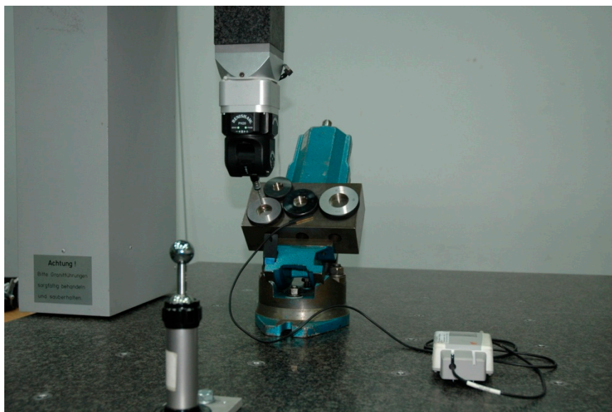
Figure 1. Five-axis measuring system and standards used during the experiments.
