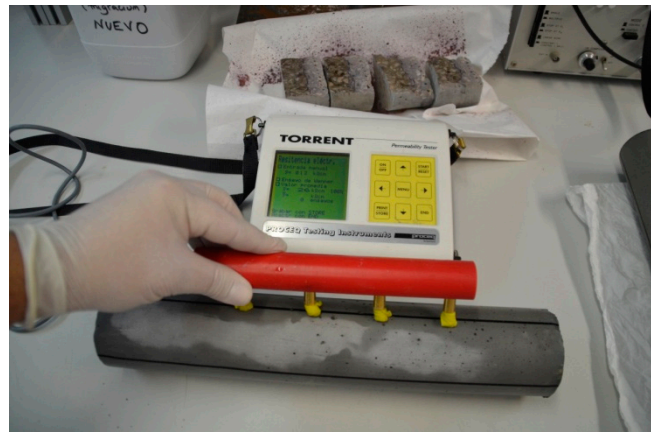
Figure 4. Electrical resistivity measurement of a 10% silica fume sample made using the four-electrode “Wenner” method.
