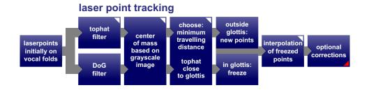
**Figure 11.** Flowchart of the laser point tracking. White corners indicate new processing steps and red corners indicate a necessary or optional user interaction.
