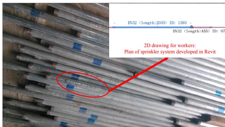
**Figure 8.** Prefabricated pipes marked with information exported from BIM model.
