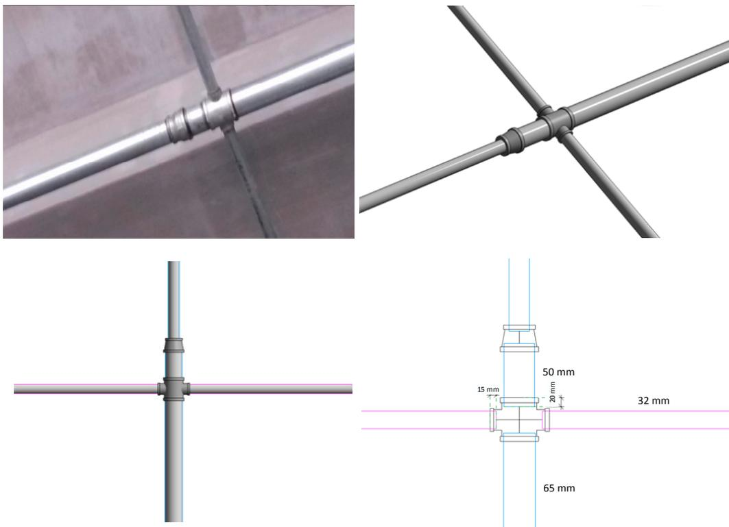
Figure 6. Detailed BIM model of a fire sprinkler system developed by the contractor.
