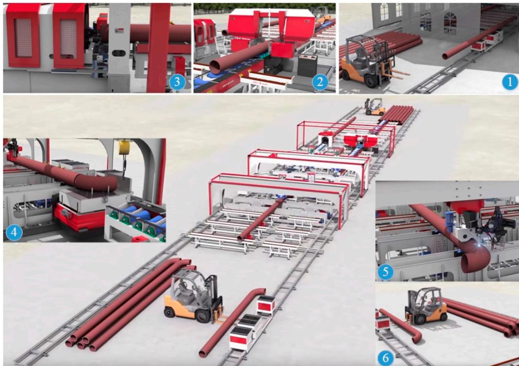
**Figure 9.** Configuration of a pipe fabrication production line. (1) the arrival of standard pipes; (2) high-speed pipe cutting machine; (3) the beveling machine; (4) the piping prefabrication fast fitting-up machine; (5) piping automatic welding machine; (6) the prefabricated pipe spools.
