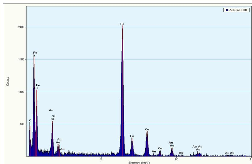
**Figure 3.** Energy dispersive X-ray (EDX) spectrum of  $\text{Fe}_3\text{O}_4/\text{Au}$  gold magnetic nanoparticles.
