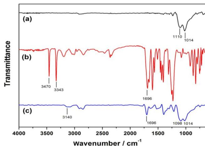
**Figure 4.** Fourier transform infrared spectroscopy (FTIR) spectra of  $\text{Fe}_3\text{O}_4/\text{Au}$  (a), 5-aminoorotic acid (AOA) (b), and  $\text{Fe}_3\text{O}_4/\text{Au-AOA}$  (c).
