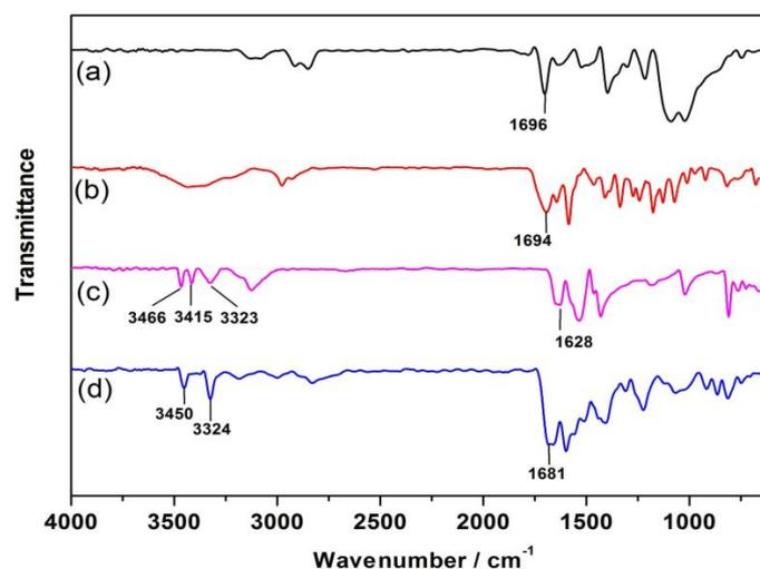
**Figure 6.** FTIR spectra of  $\text{Fe}_3\text{O}_4/\text{Au- AOA}$  (a),  $\text{AOA-RhB}$  (b), melamine (c), and  $[\text{Fe}_3\text{O}_4/\text{Au- AOA} \bullet \bullet \bullet \text{melamine} \bullet \bullet \bullet \text{AOA-RhB}]$  (d).
