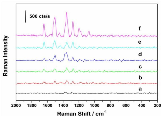
**Figure 9.** Raman spectra of  $[\text{Fe}_3\text{O}_4/\text{Au-AOA}\bullet\bullet\bullet\text{melamine}\bullet\bullet\bullet\text{AOA-RhB}]$  in milk at melamine concentration of 0  $\mu\text{g/mL}$  (a), 2.0  $\mu\text{g/mL}$  (b), 2.5  $\mu\text{g/mL}$  (c), 5.0  $\mu\text{g/mL}$  (d), 10.0  $\mu\text{g/mL}$  (e), and 15.0  $\mu\text{g/mL}$  (f).
