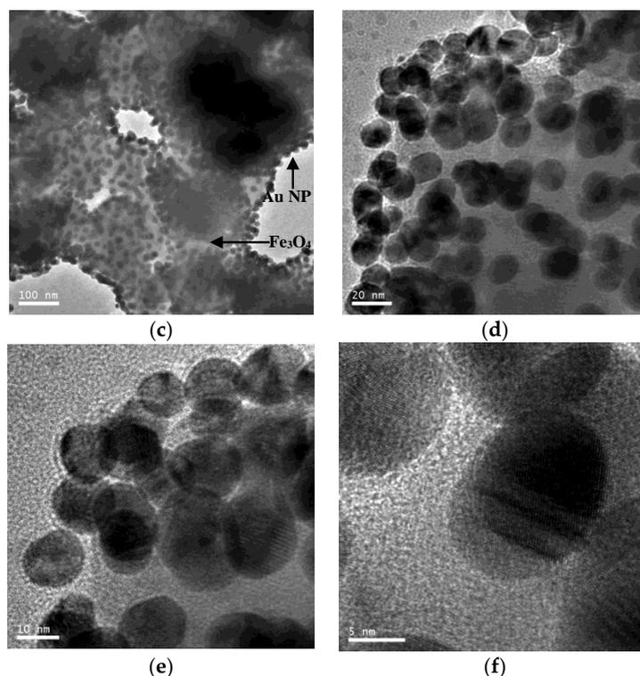
**Figure 2.** Transmission electron microscope (TEM) images of  $\text{Fe}_3\text{O}_4$  nanoparticles (a), Au nanoparticles (b),  $\text{Fe}_3\text{O}_4/\text{Au}$  nanoparticles at normal resolution (c–e), and high resolution (f).
