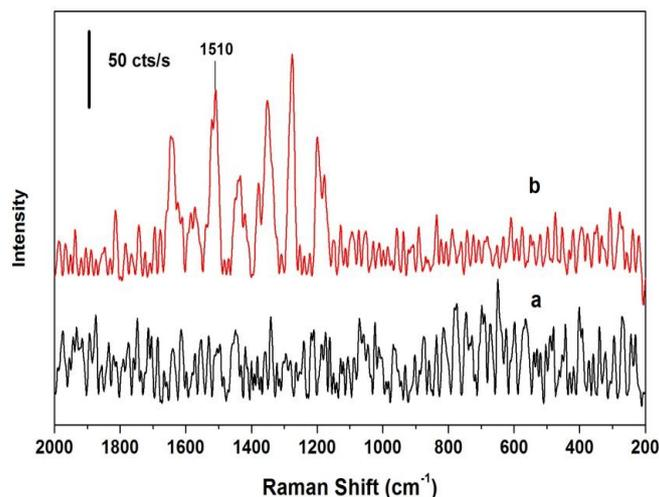
**Figure 7.** Raman spectra of the mixture of  $\text{Fe}_3\text{O}_4/\text{Au-AOA}$  and  $\text{AOA-RhB}$  (a) in the absence of melamine and (b) in the presence of  $1.0 \mu\text{g/mL}$  of melamine.
