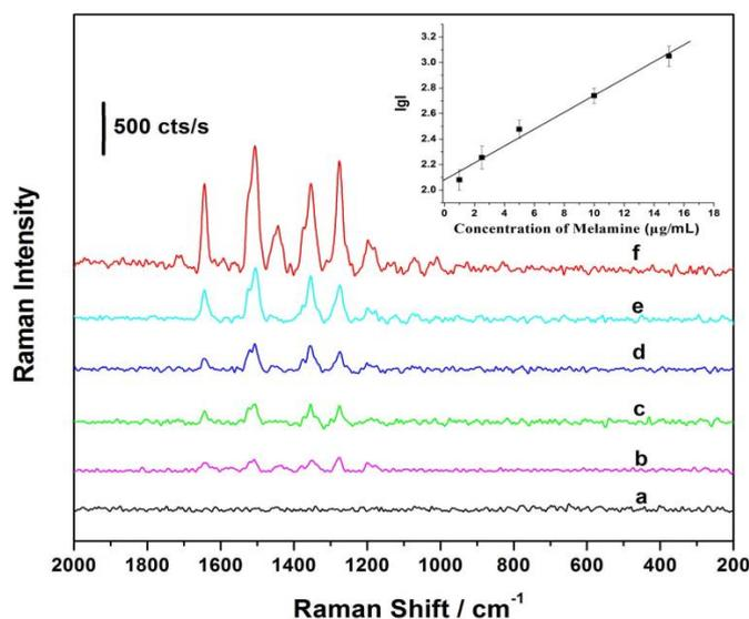
**Figure 8.** Raman spectra of  $[\text{Fe}_3\text{O}_4/\text{Au-AOA}\bullet\bullet\bullet\text{melamine}\bullet\bullet\bullet\text{AOA-RhB}]$  in water at melamine concentration of  $0 \mu\text{g/mL}$  (a),  $1.0 \mu\text{g/mL}$  (b),  $2.5 \mu\text{g/mL}$  (c),  $5.0 \mu\text{g/mL}$  (d),  $10.0 \mu\text{g/mL}$  (e), and  $15.0 \mu\text{g/mL}$  (f). (Inset: logarithmic linear correlation of peak intensity at  $1510 \text{ cm}^{-1}$  and melamine concentrations).
