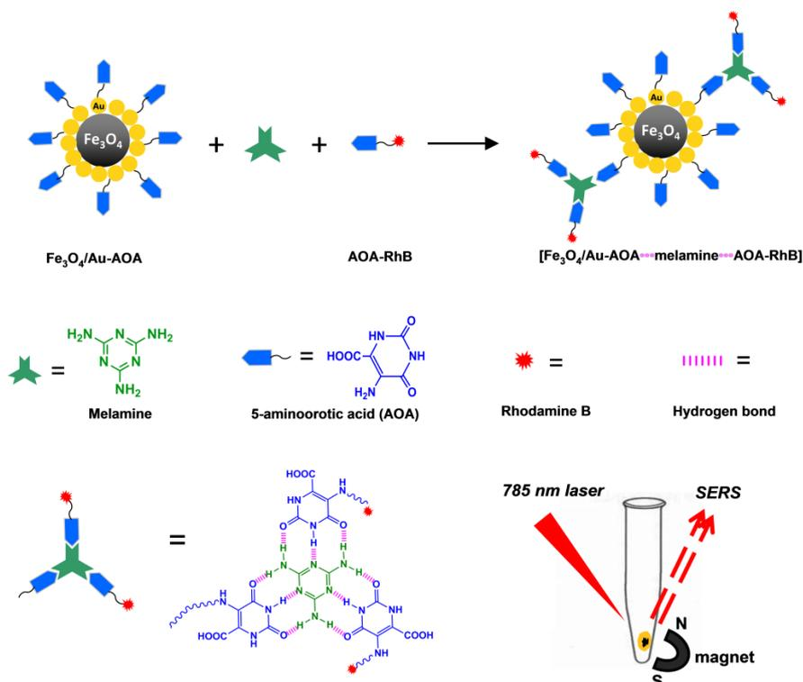
**Figure 1.** The hydrogen bonding-assisted  $[\text{Fe}_3\text{O}_4/\text{Au-AOA}\cdots\text{melamine}\cdots\text{AOA-RhB}]$  surface enhanced Raman spectroscopy (SERS) matrix.
