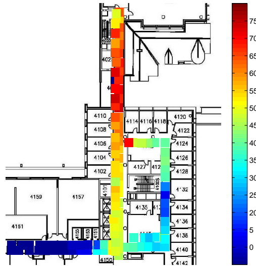
Figure 2. RSS values of an AP over the corridor area of the fourth floor of the Bahen Building, University of Toronto.
