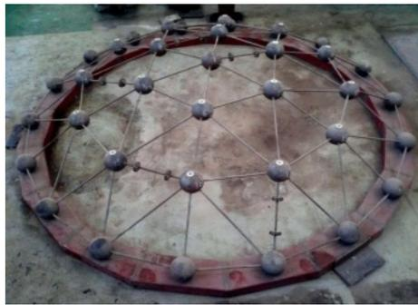
Figure 3. Photo of test model of the K6 single-layer spherical shell.
