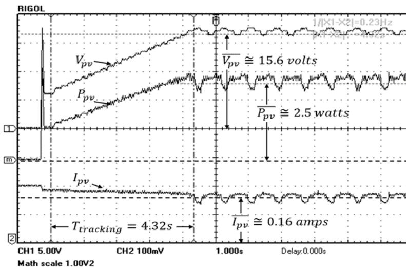
Figure 23. The performance of the proposed fuzzy logic-based algorithm.
