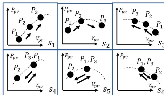
Figure 3. P and O: movement locus of the PV operation point.
