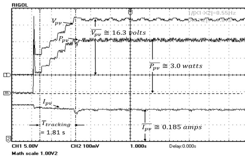
Figure 22. The performance of the conventional P and O algorithm.
