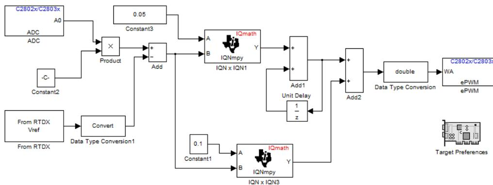
Figure 19. MATLAB/Simulink diagram of the PI controller.
