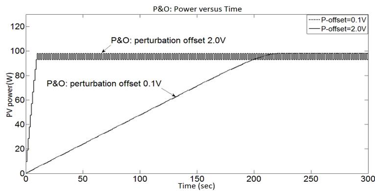
Figure 5. P and O: tracking traces with different perturbation offsets.
