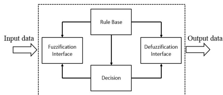
Figure 8. The structure of a fuzzy logic controller.
