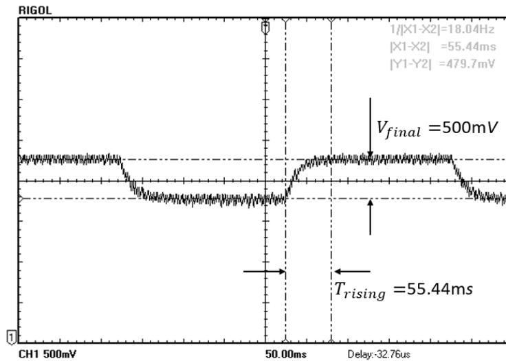
Figure 20. The step response of the inner control loop of the PV system.
