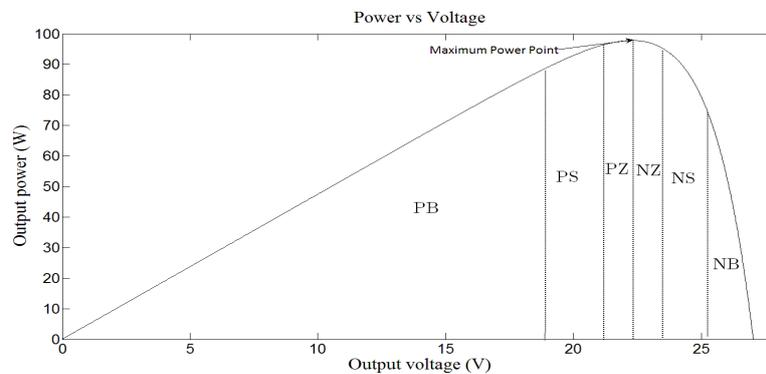
Figure 7. A sectionalized P-V curve.
