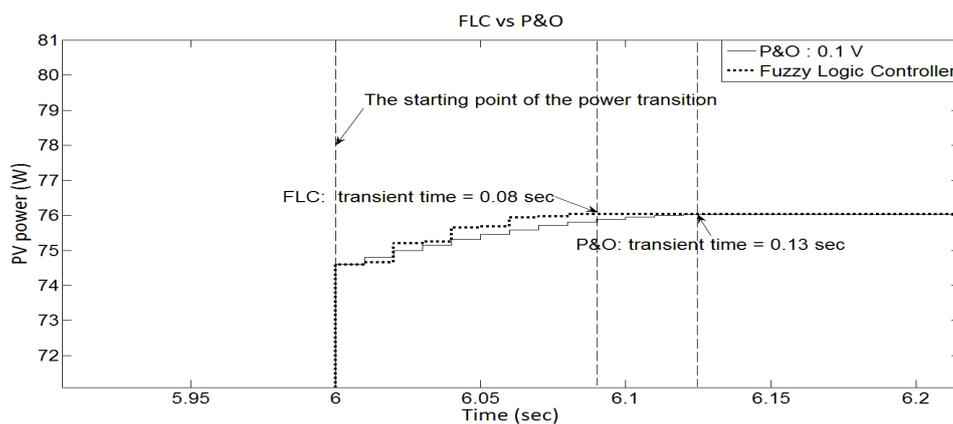
Figure 16. Second transition caused by the irradiation increasing.
