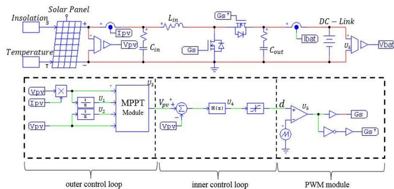
Figure 6. The general structure of PV MPPT system in a power converter.
