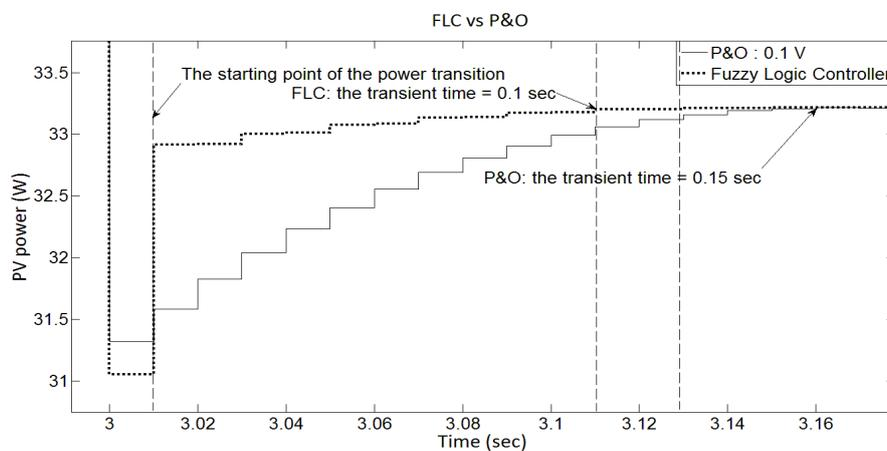
Figure 15. First transition caused by the irradiation drop.
