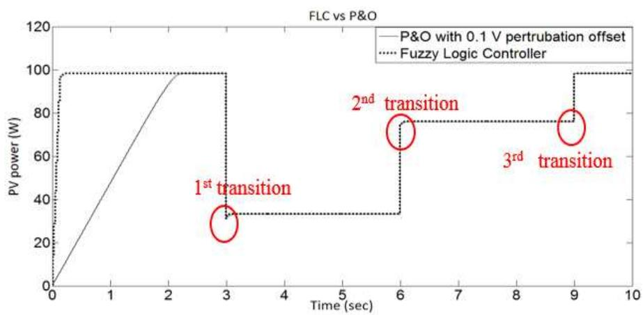
Figure 13. The proposed algorithm (FLC) vs. the conventional P and O algorithm.
