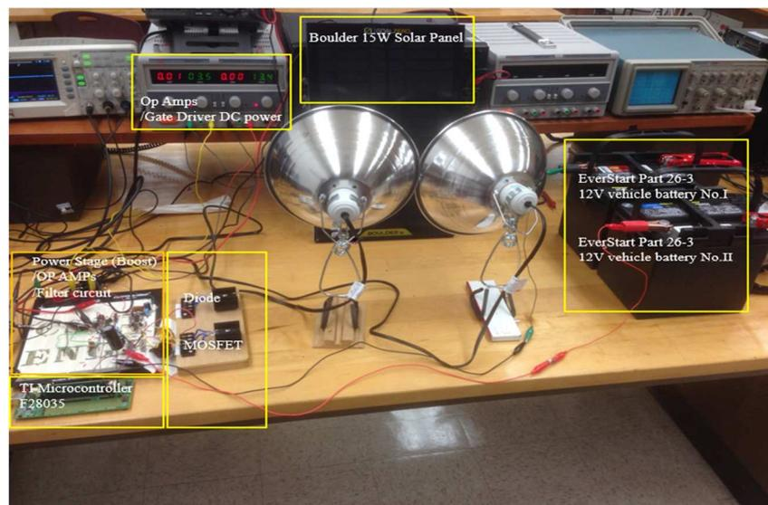
Figure 21. The experimental setup of the photovoltaic system.
