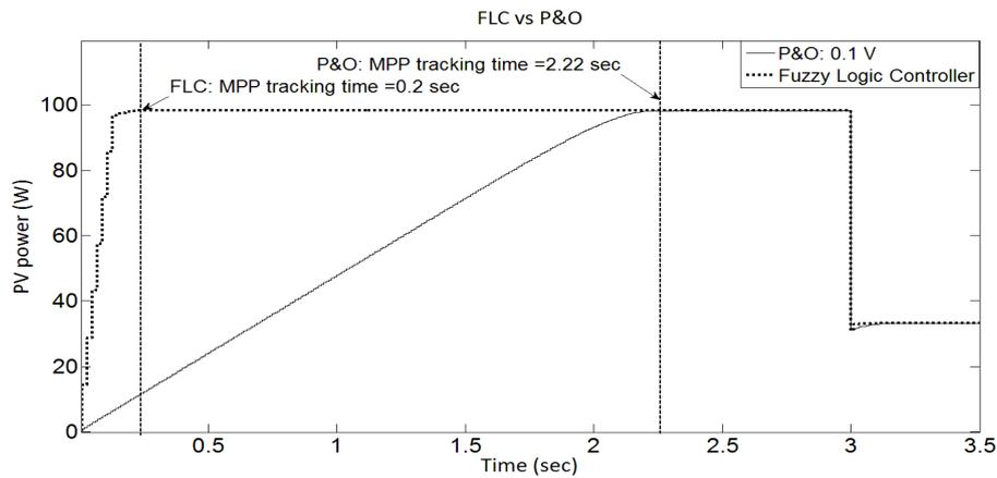
Figure 14. Initial tracking time: FLC vs. P and O (0.1 V).
