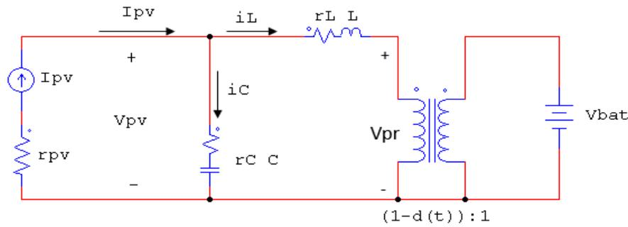
Figure 18. The small signal model of the input terminal.
