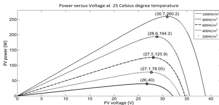
Figure 2. P-V cruves of SW-260-mono operating.
