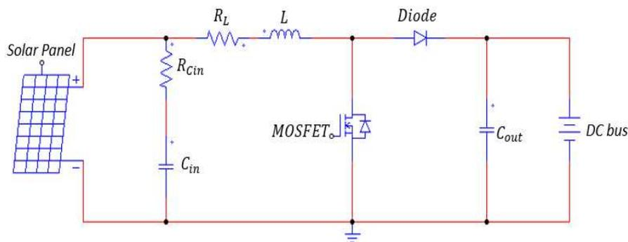
Figure 17. The topology of the photovoltaic boost DC-DC converter.
