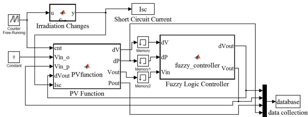
**Figure 10.** The MATLAB/Simulink diagrams of the FLC.
