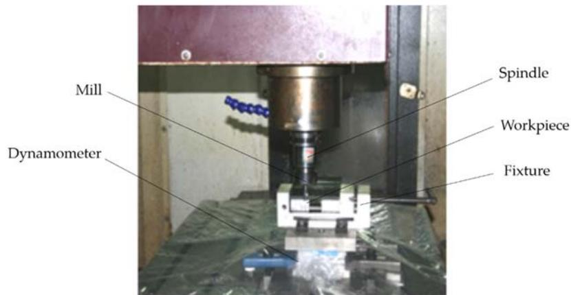
Figure 7. Experimental setup.
