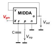
**Figure 8.** Simple application of a proposed MIDDA in a first-order high-pass filter with adjustable pole frequency.
