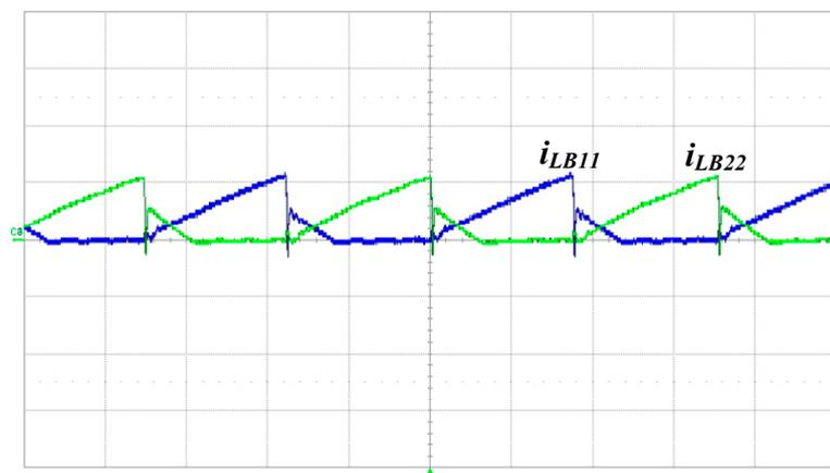
**Figure 8.** Measured coupled inductor currents  $i_{LB11}$  (2 A/div) and  $i_{LB22}$  (2 A/div); time scale: 5  $\mu$ s/div.
