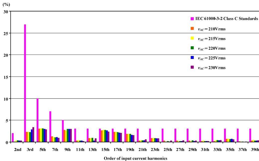
Figure 15. Measured input current harmonics compared with the IEC 61000-3-2 Class C standards.
