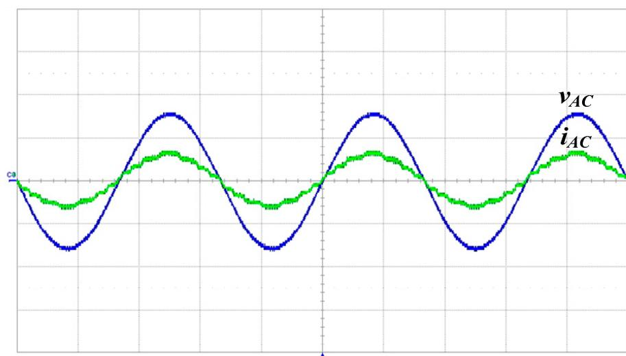
Figure 14. Measured input utility-line voltage  $v_{AC}$  (200 V/div) and current  $i_{AC}$  (2 A/div); time scale: 5 ms/div.
