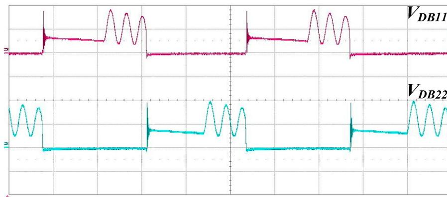
Figure 13. Measured voltages on the diodes  $D_{B11}$  and  $D_{B22}$ . Voltage scale: 200 V/div; time scale: 5  $\mu$ s/div.
