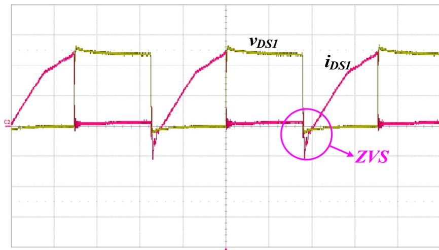
Figure 9. Measured switch voltage  $v_{DS1}$  (200 V/div) and current  $i_{DS1}$  (2 A/div); time scale: 5  $\mu$ s/div.
