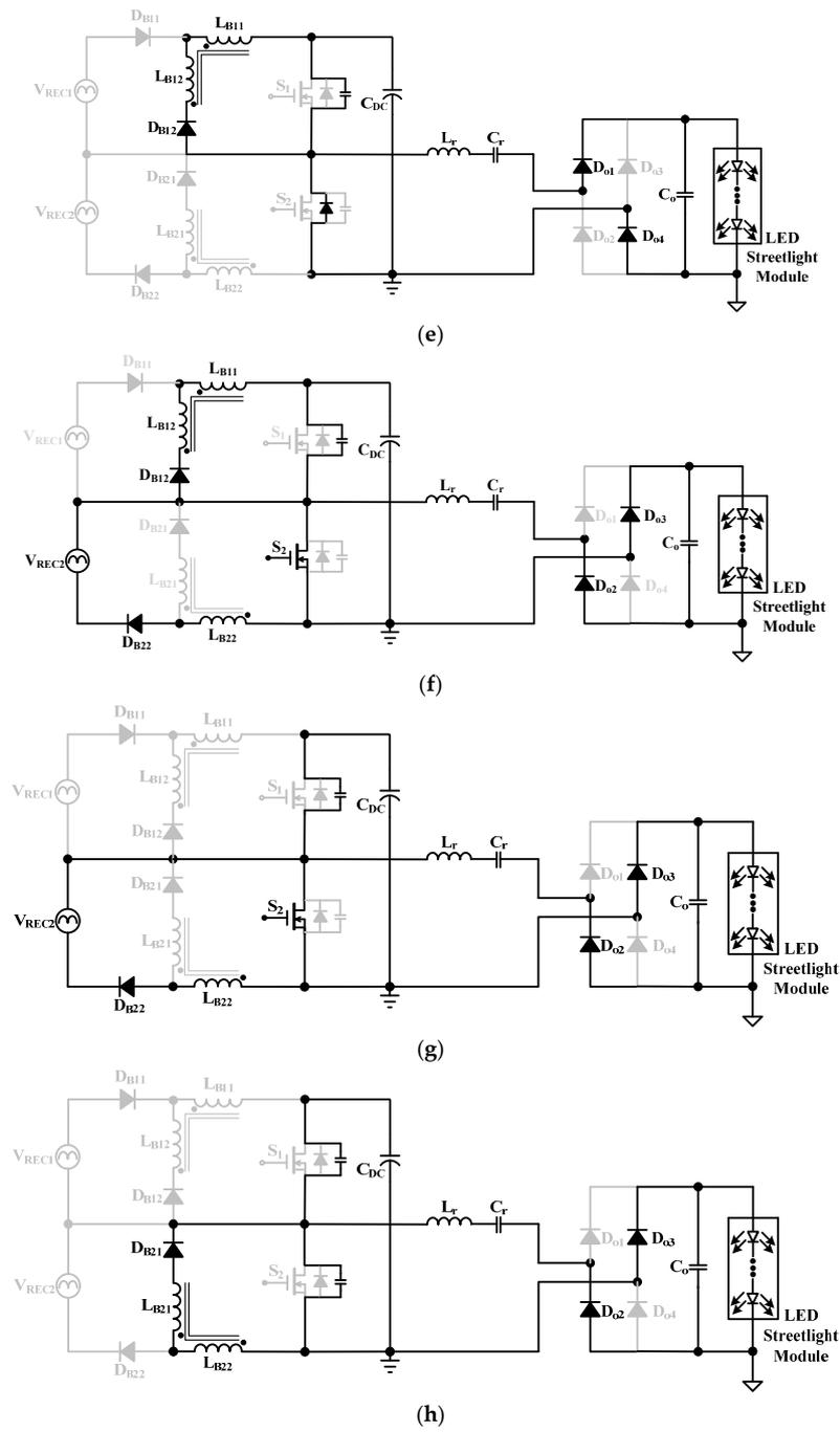
**Figure 5.** Operation modes of the presented LED driver; (a) Model 1; (b) Model 2; (c) Model 3; (d) Model 4; (e) Model 5; (f) Model 6; (g) Model 7; (h) Model 8.
