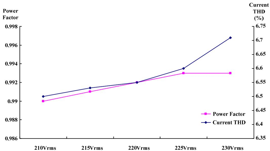
Figure 16. Measured power factor and current total harmonic distortion (THD) under utility-line voltages ranging from 210 to 230 V.
