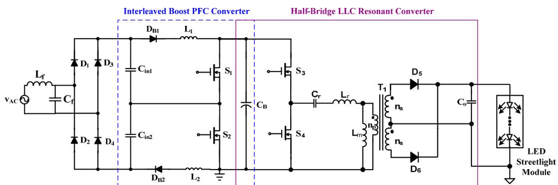
**Figure 1.** The conventional two-stage light-emitting diode (LED) driver for streetlighting applications, PFC: power factor correction.
