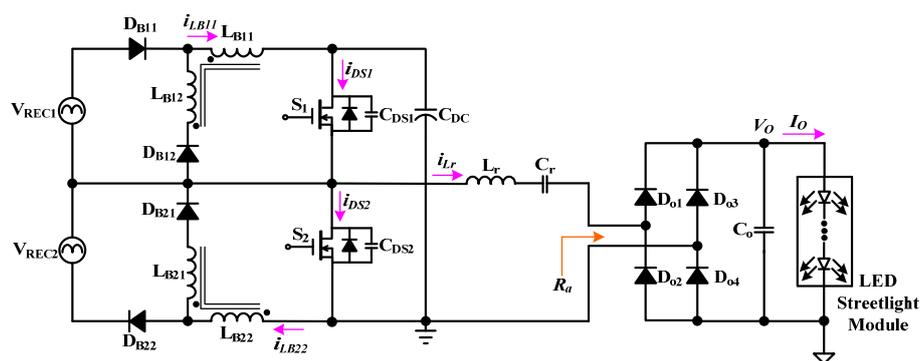
Figure 4. Simplified circuit of the presented single-stage LED driver for streetlight applications.
