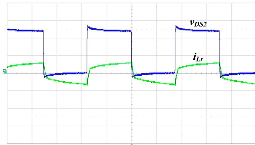
Figure 11. Measured switch voltage  $v_{DS2}$  (200 V/div) and resonant inductor current  $i_{Lr}$  (2 A/div); time scale: 5  $\mu$ s/div.
