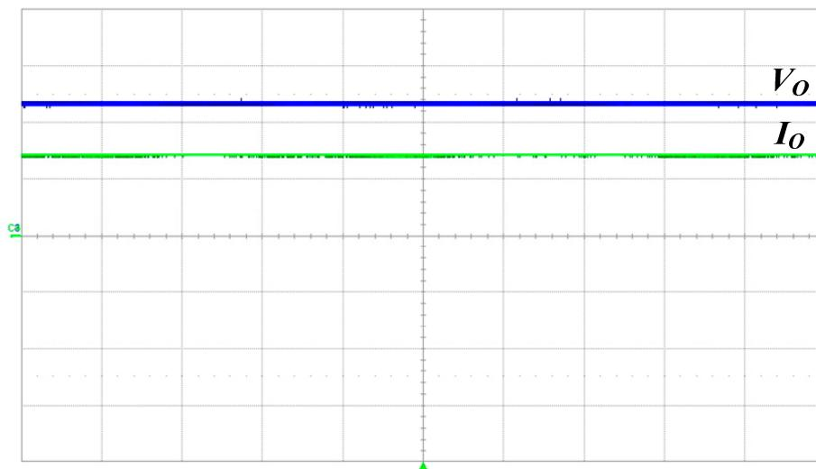
Figure 12. Measured output current  $I_O$  (0.5 A/div) and voltage  $V_O$  (100 V/div); time scale: 2 ms/div.
