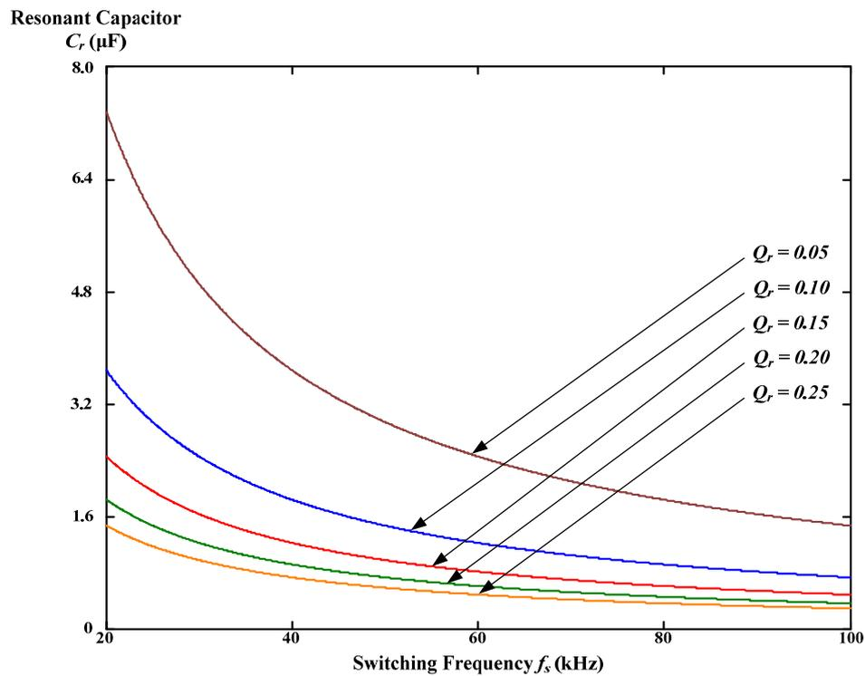
**Figure 7.** Resonant capacitor  $C_r$  versus the switching frequency  $f_s$  under different levels of quality factor  $Q_r$ .
