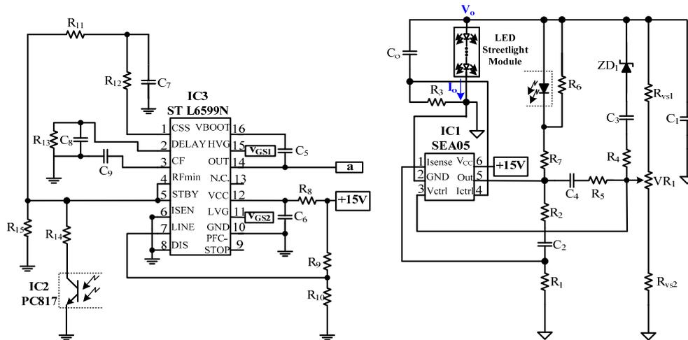
Figure 3. The utilized control circuit of the presented single-stage LED driver for streetlight applications.
