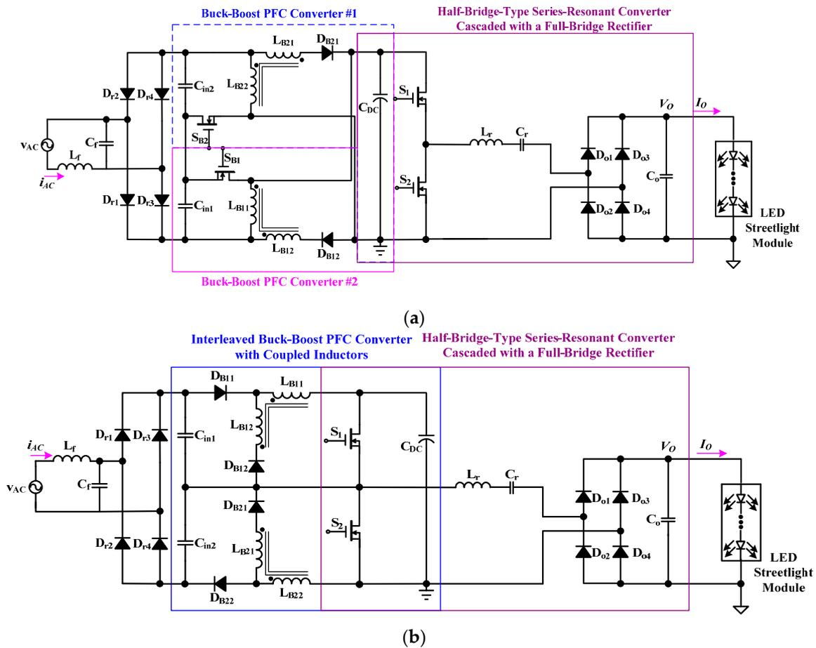
Figure 2. (a) Original two-stage LED driver circuit; (b) the presented single-stage LED driver with coupled inductors and interleaved PFC for streetlight applications.
