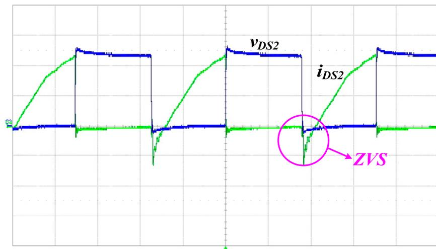
Figure 10. Measured switch voltage  $v_{DS2}$  (200 V/div) and current  $i_{DS2}$  (2 A/div); time scale: 5  $\mu$ s/div.
