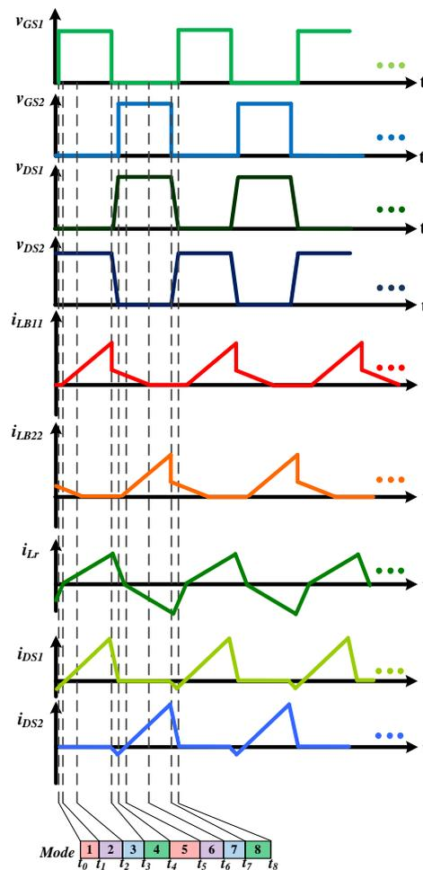
Figure 6. Key waveforms of the presented LED driver for streetlight applications.
