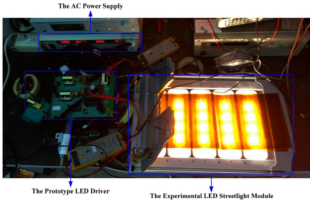
**Figure 18.** Photograph of supply of the experimental LED streetlight module using the presented driver at a utility-line voltage of 220 V, AC: Alternating-Current.
