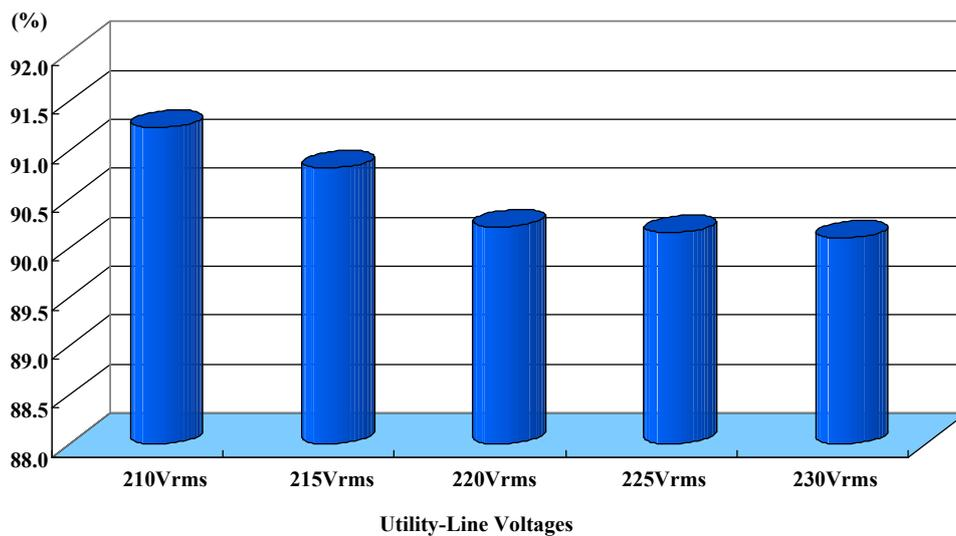
Figure 17. Measured circuit efficiency under utility-line voltages ranging from 210 to 230 V.
