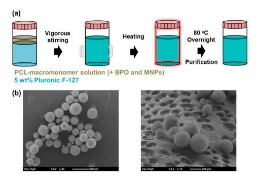
**Figure 1.** (a) Schematic illustration of preparation procedure of shape-memory PCL microparticles by in-situ oil-in-water (o/w) emulsion polymerization technique; (b) Top view (Left) and tilt view (Right) SEM images of prepared shape-memory PCL microparticles with acceleration voltage of 5 kV. Scale bars, 500  $\mu$ m (Left) and 200  $\mu$ m (Right).
