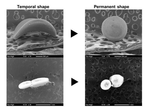
**Figure 3.** SEM images of thermally-induced shape recovery of shape-memory PCL microparticles with acceleration voltage of 5 kV (**top**) and 10 kV (**bottom**). Highly strained temporary shape (**left**) was returned to original permanent shape (**right**) by heating at 37 °C for 15 min. Images shows the shape recovery of particles for two different sets (**top** and **bottom**). Scale bars, 200  $\mu$ m (**top**) and 1 mm (**bottom**).
