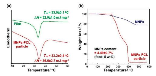
**Figure 2.** (a) DSC curves of shape-memory PCL microparticles containing MNPs and crosslinked PCL film as a control. The  $T_{\rm m}$  and  $\Delta H$  were estimated from peak top and area of endothermic peak, respectively; (b) Thermogravimetric analysis for MNPs as a control and shape-memory PCL microparticles containing MNPs.
