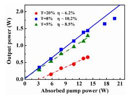
Figure 2. Continuous-wave (CW) output power vs. absorbed pump power with different output couplers.
