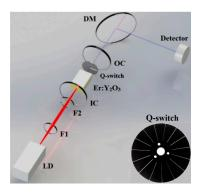
**Figure 1.** Schematic setup of the Q-switched Er:Y<sub>2</sub>O<sub>3</sub> ceramic laser. LD: laser diode; IC: input coupler; OC: output coupler; DM: dichroic mirror.
