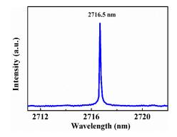
Figure 7. Spectrum of the Q-switched Er:Y<sub>2</sub>O<sub>3</sub> laser.
