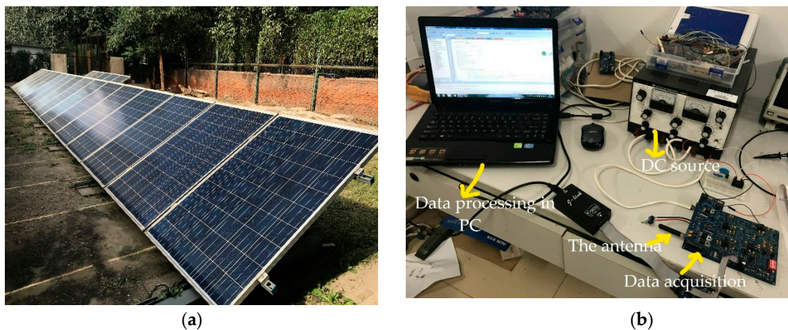
Figure 6. The experimental platform. (a) The experimental photovoltaic system; (b) The experimental instrument. DC: Direct Current.
