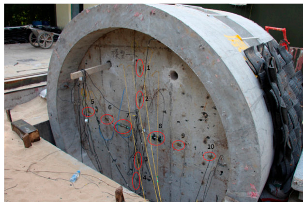
Figure 22. Reinforced concrete specimen with FBGs without coating and other FBG sensors.
