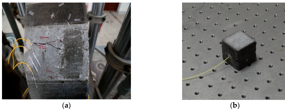
Figure 2. Samples of polyimide FBGs. (a) Cracking monitoring with bare FBGs; (b) A similar material sensor with bare FBGs.
