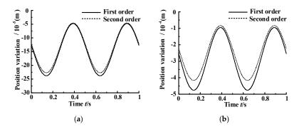
**Figure 12.** Position variation resulting from  $K_D$  variation. (**a**) Four parameters increase 10%; (**b**) Four parameters increase 20%.
