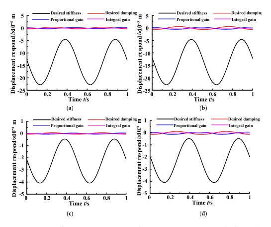
**Figure 17.** Variation of position response when each parameter increases 10%. (**a**) The first working condition; (**b**) The second working condition; (**c**) The third working condition; (**d**) The fourth working condition.
