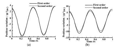
**Figure 14.** Position variation resulting from  $K_P$  variation. (**a**) Four parameters increase 10%; (**b**) Four parameters increase 20%.
