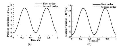
**Figure 13.** Position variation resulting from  $C_D$  variation. (a) Four parameters increase 10%; (b) Four parameters increase 20%.
