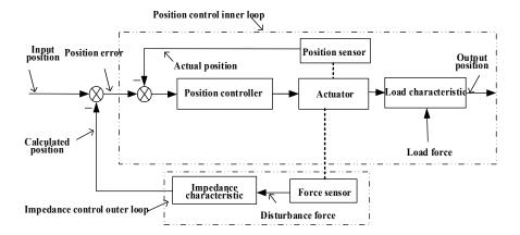
Figure 6. Position-based impedance control schematic.
