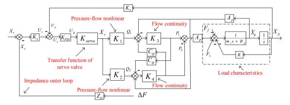
Figure 7. Block diagram of HDU position-based impedance control.
