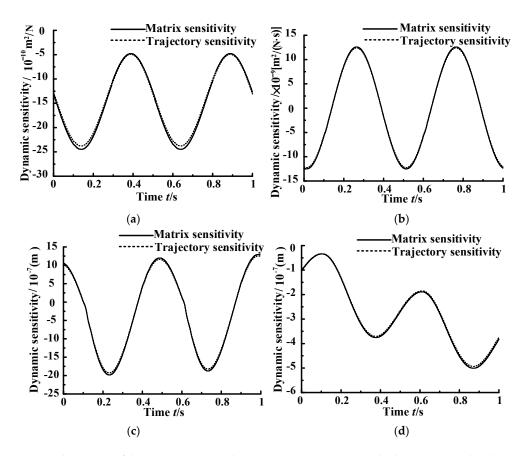
**Figure 16.** The curves of dynamic sensitivity between two sensitivity methods. (a) First-order dynamic sensitivity of  $K_D$ ; (b) First-order dynamic sensitivity of  $C_D$ ; (c) First-order dynamic sensitivity of  $K_p$ ; (d) First-order dynamic sensitivity of  $K_i$ .
