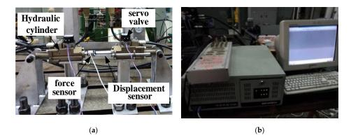
**Figure 3.** Composition of HDU performance test platform. (a) HDU performance test platform; (b) dSPACE controller.
