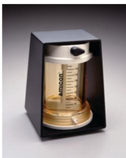
**Figure 1.** Transparent plastic dead-end cell (Amicon, Denver, MA, USA, model 8200).
